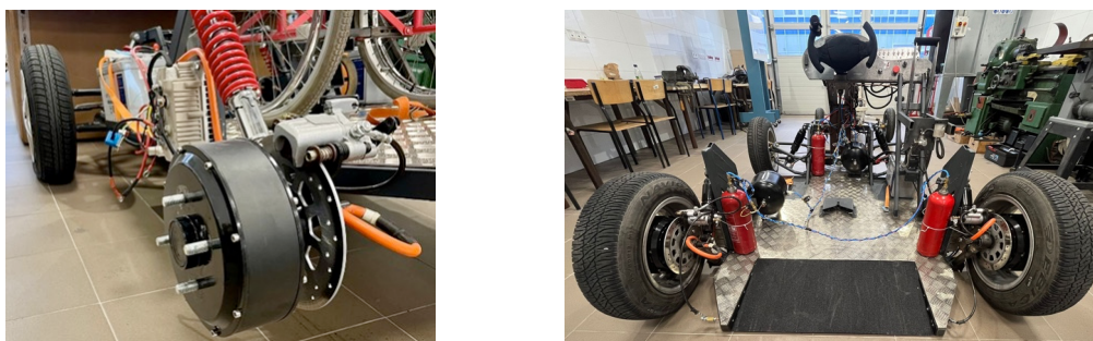
Fig. 4. BLDC motor mounted directly on the test vehicle
