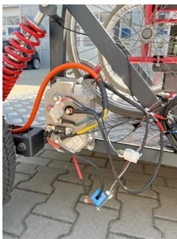
Fig. 6. LEM HAIS 100-A current sensor installed in the test vehicle
