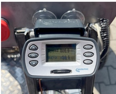
Fig. 5. Racelogic device mounted on the vehicle during testing
