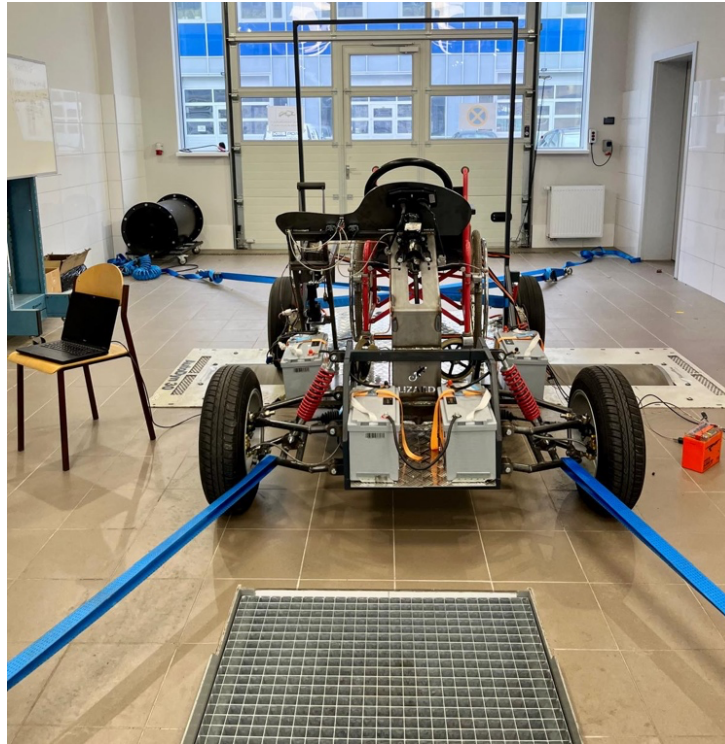
Fig. 8. Testing the four-wheeler on an AutoDyn 30 chassis dynamometer
