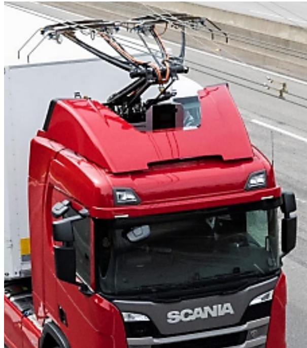
Fig. 5. The current collector of a freight vehicle with a contact network
