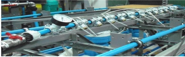
Fig. 5. System used for testing individual measuring channels with the visible joints for installation of pressure sensors
