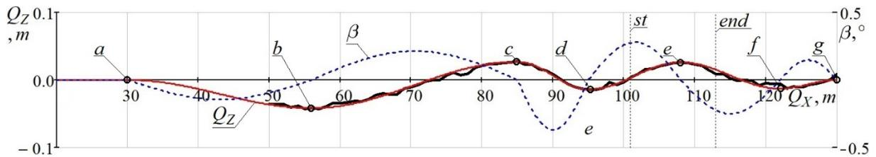
Fig. 5. Vertically enlarged (100 times) depiction of the longitudinal profile of the road surface of the bridge crossing, the dependence of its vertical coordinate  $Q_Z$ , and the longitudinal angle  $\beta$  on the longitudinal coordinate  $Q_X$
