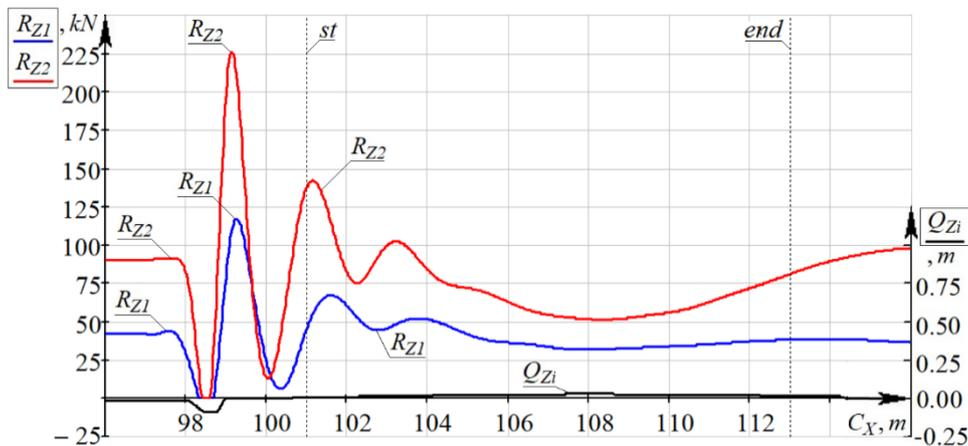
Fig. 11. Dependencies of the vertical reactions of the road surface of the bridge crossing on the wheels of the front  $R_{Z1}$  and rear  $R_{Z2}$  axles of the truck on the longitudinal coordinate of its center of sprung masses  $C_X$  in the area of overcoming the pothole and the bridge
