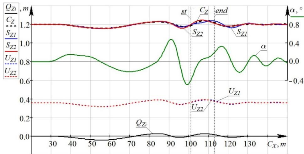
Fig. 7. Dependencies of the vertical coordinates of the center of sprung masses  $C_Z$  of a truck, brought to its front wheels  $S_{Z1}$  and rear  $S_{Z2}$  axles of equivalent sprung masses, unsprung masses  $U_{Z1}$  and  $U_{Z2}$ , as well as pitch angle  $\alpha$  from the longitudinal coordinate of the center of sprung masses  $C_X$
