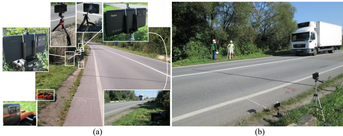
Fig. 3. Places of installation of video cameras (a) to capture the nature of the movement of the MAN TGL 12.220 truck (b) while crossing the bridge crossing
