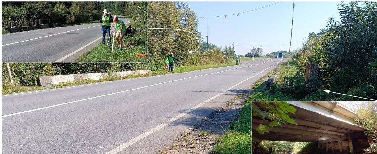
Fig. 1. Leveling of the road pavement profile of the bridge with a step of 1 m
