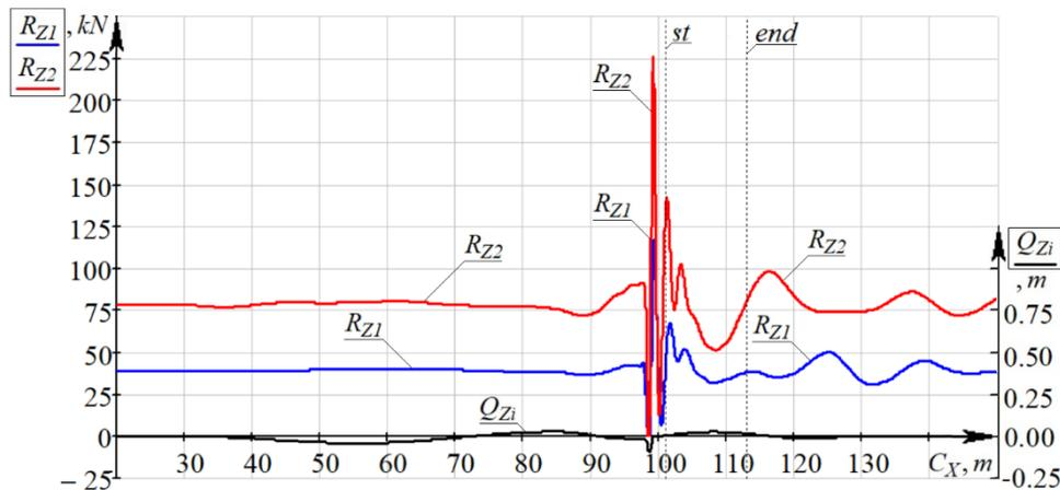
Fig. 10. Dependencies of the vertical reactions of the road surface of the bridge crossing on the wheels of the front  $R_{Z1}$  and rear  $R_{Z2}$  axles of the truck on the longitudinal coordinate of its center of sprung masses  $C_X$
