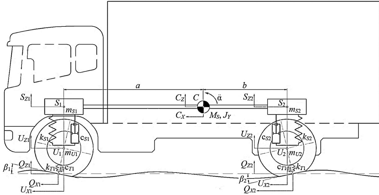
Fig. 4. Half-car model of the dynamics of the truck movement across the bridge crossing
