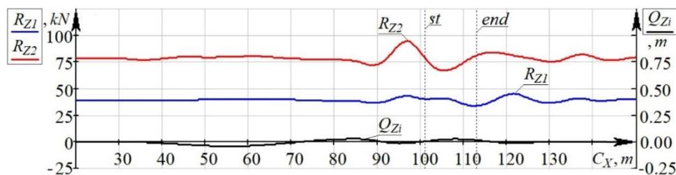
Fig. 8. Dependencies of the vertical reactions of the road surface of the bridge crossing on the wheels of the front  $R_{Z1}$  and rear  $R_{Z2}$  axles of the truck on the longitudinal coordinate of its center of sprung masses  $C_X$
