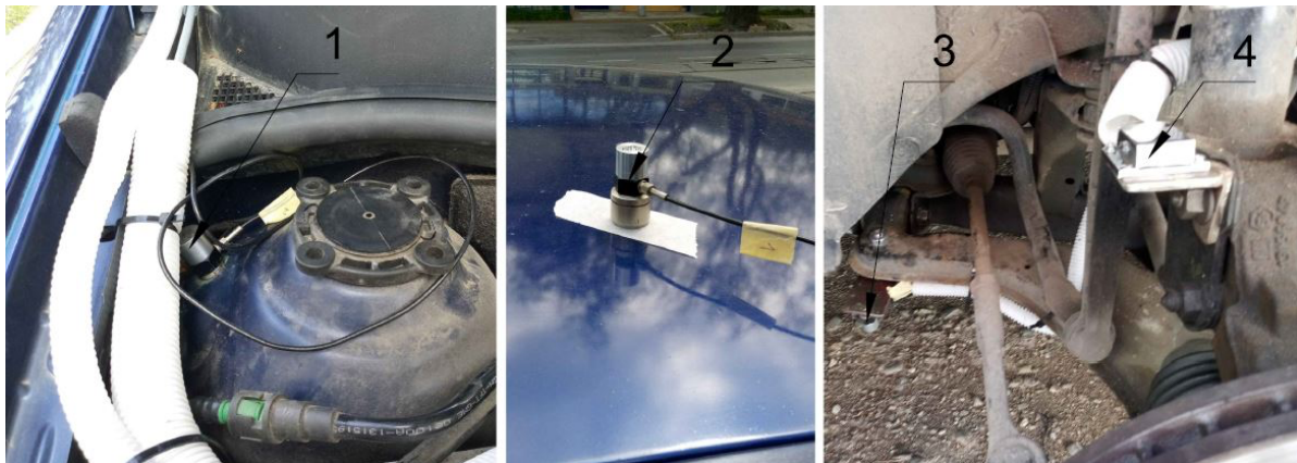
Fig. 2. Location of the measuring points: 1 – on the body, 2 – on the roof, 3 – on the control arm, and 4 – on the wheel hub carrier
