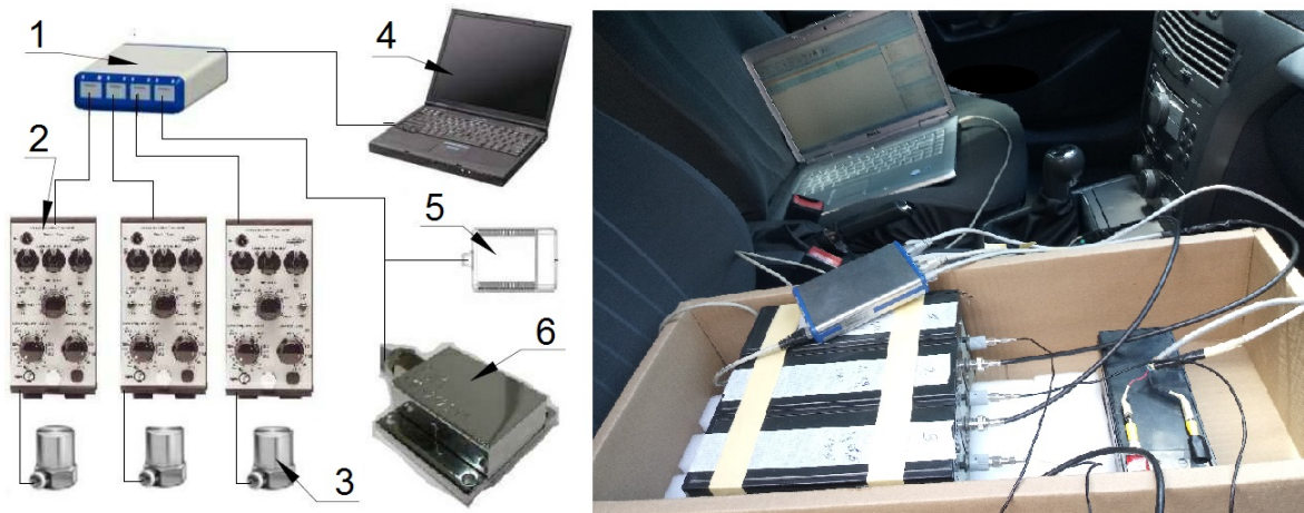
Fig. 3. Setup of the measuring system: 1 – DAQ system, 2 – charge amplifiers, 3 – piezoelectric accelerometers, 4 – laptop, 5 – 12V battery, 6 – capacitive accelerometer
