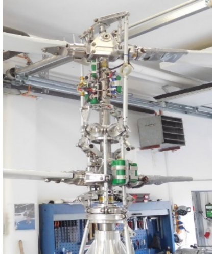
Fig. 2. Measuring equipment on the coaxial rotor system
