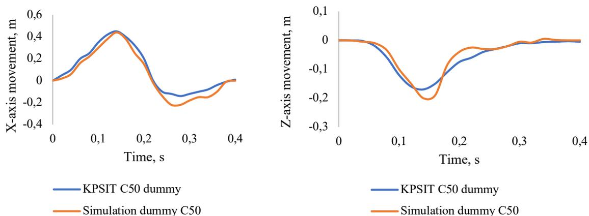
Fig. 1. Illustration of head movement along the X and Z axes for the physical and the simulation dummy during a frontal collision
