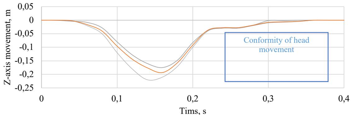
Fig. 18. Head Position Changes (Z-axis) for Dummy and Volunteers - Frontal Crash with Three-point Seat Belts Passenger Vehicle Seat
