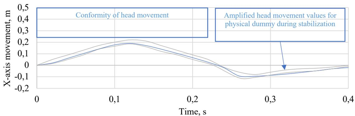
Fig. 15. Head Position Changes (X-axis) for Dummy and Volunteers - Frontal Crash with Four-point Belts Sports Bucket Seat
