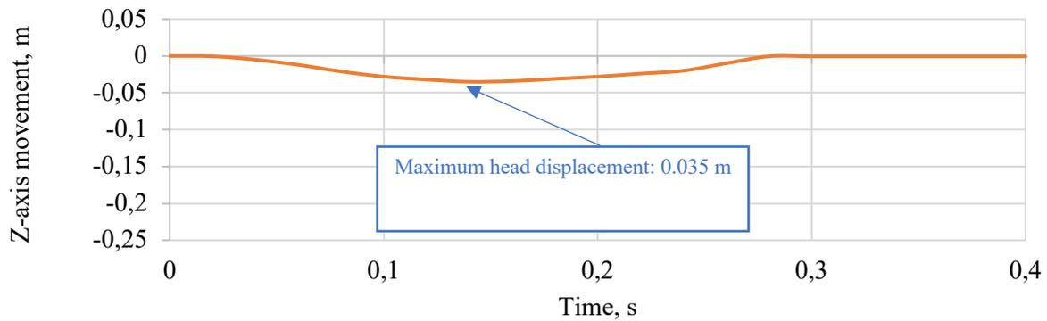
Fig. 12. Head Position Shift (Z-axis) for C50 Volunteers - Four-point Belts Sports Bucket Seat
