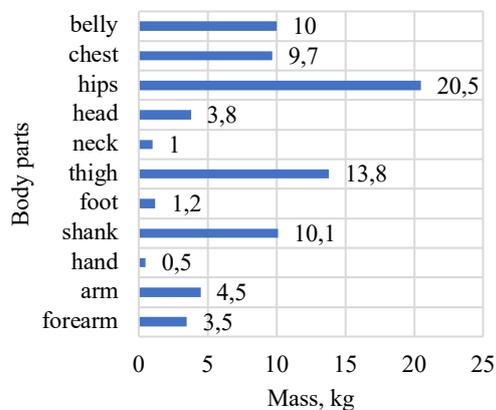
Fig. 2. Mass of the components of the physical KPSIT dummy C50
