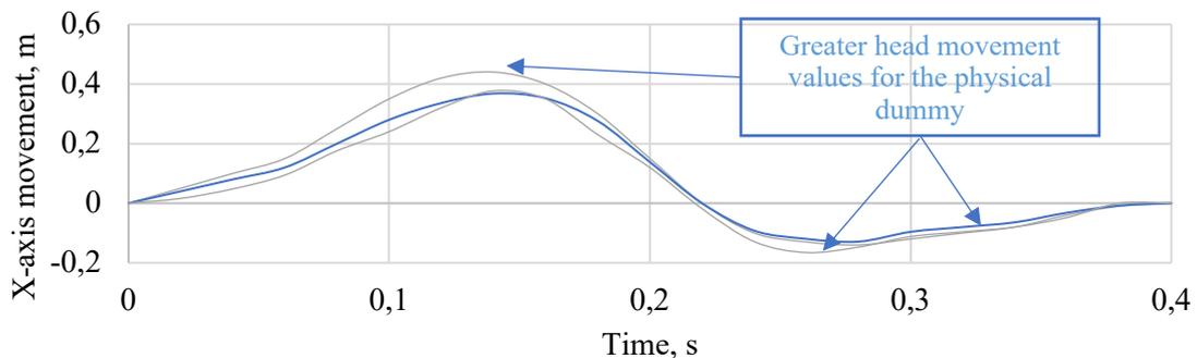
Fig. 17. Head Position Changes (X-axis) for Dummy and Volunteers - frontal crash with three-point seat belts passenger vehicle seat
