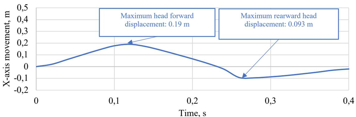
Fig. 11. Head Position Shift (X-axis) for C50 Volunteers - Four-point Belts Sports Bucket Seat
