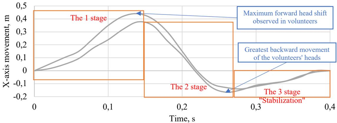
Fig. 9. Head Position Shift (X-axis) for C50 Volunteers - Passenger Vehicle Seat
