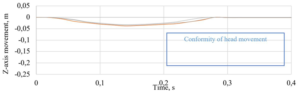
Fig. 16. Head Position Changes (Z-axis) for Dummy and Volunteers - Frontal Crash with Four-point Belts Sports Bucket Seat
