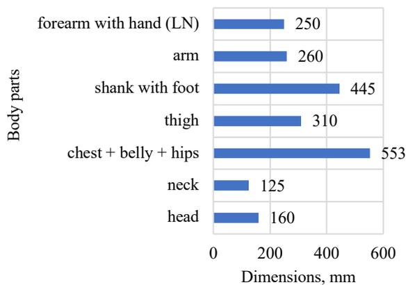
Fig. 3. Dimensions of the elements of the physical KPSIT dummy C50
