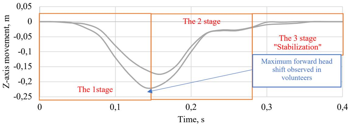
Fig. 10. Head Position Shift (Z-axis) for C50 Volunteers - Passenger Vehicle Seat
