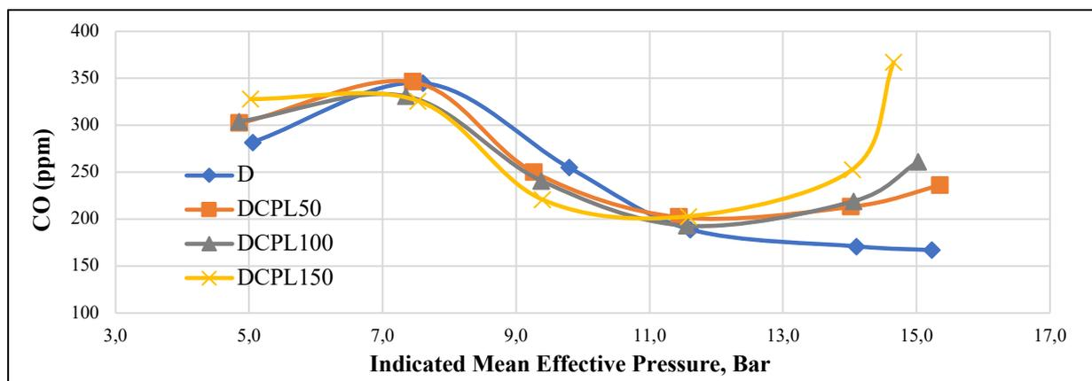
Fig. 7. Influence of nanoparticle content in diesel on CO emissions
