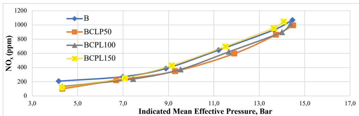
Fig. 6. Influence of nanoparticle content in biodiesel on NO<sub>x</sub> emissions
