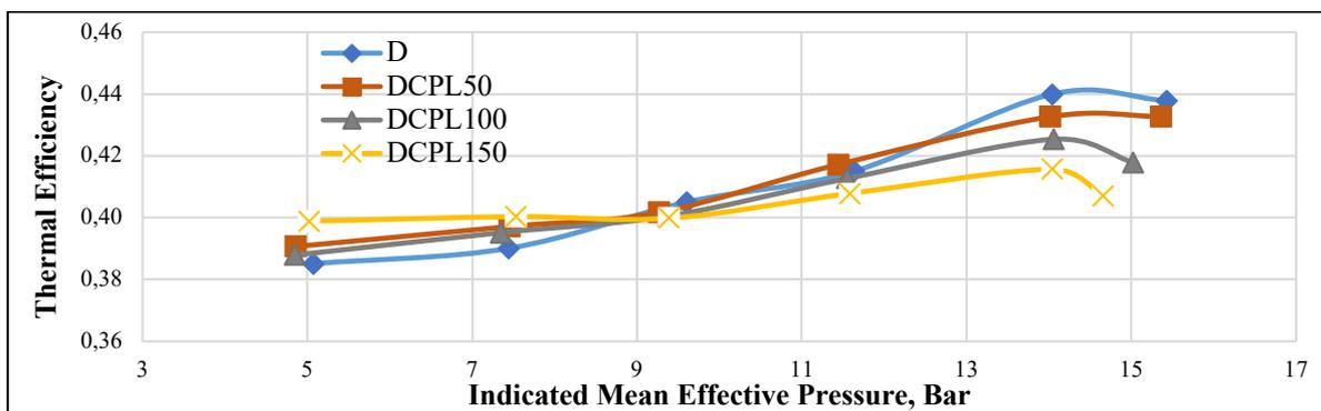
Fig. 3. Influence of nanoparticle content in diesel fuel on thermal efficiency
