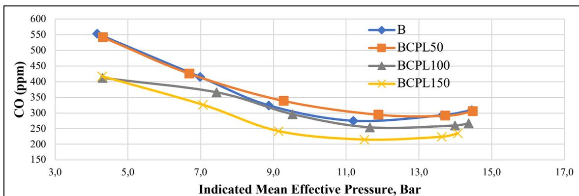
Fig. 8. Influence of nanoparticle content in biodiesel on CO emissions
