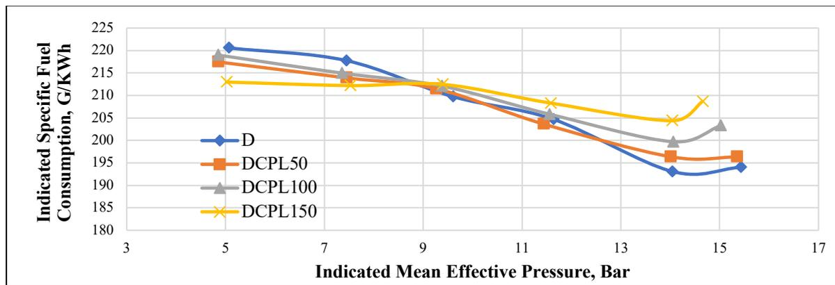
Fig. 1. Influence of nanoparticle content in diesel fuel on indicated specific fuel consumption
