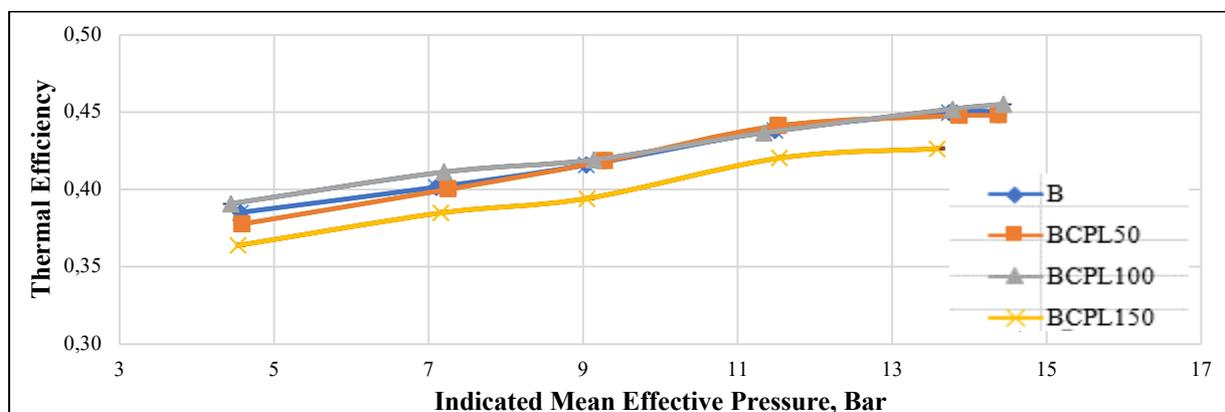
Fig. 4. Influence of nanoparticle content in biodiesel fuel on thermal efficiency
