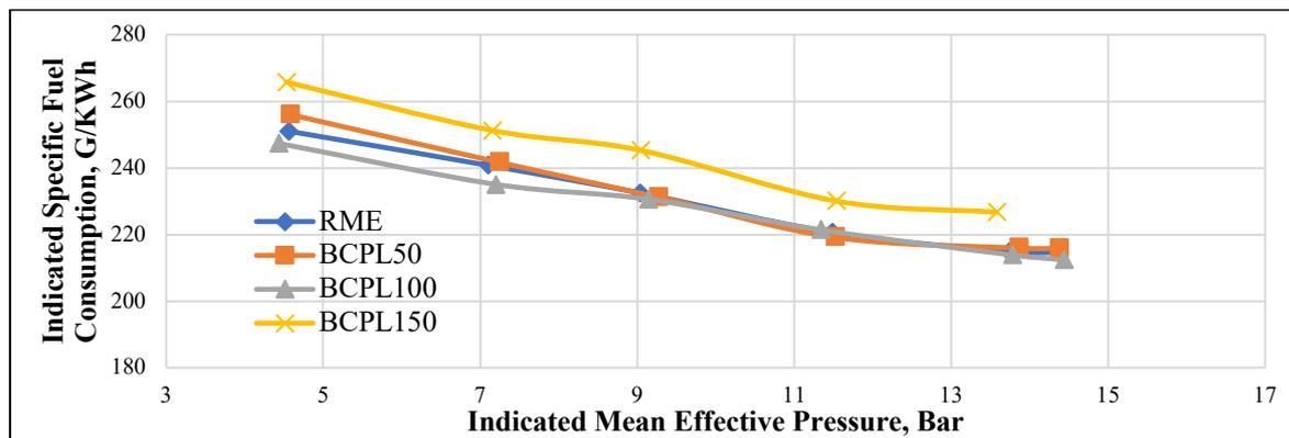
Fig. 2. Influence of nanoparticle content in biodiesel fuel on indicated specific fuel consumption
