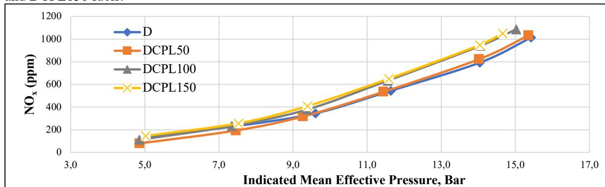
Fig. 5. Influence of nanoparticle content in diesel fuel on NO<sub>x</sub> emissions
