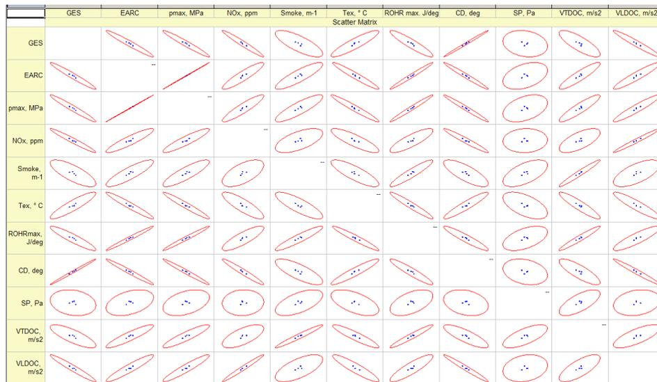
Fig. 2. Vibration and sound pressure correlations with engine parameters. *BMEP*: 0.3 MPa. Pilot fuel: diesel
