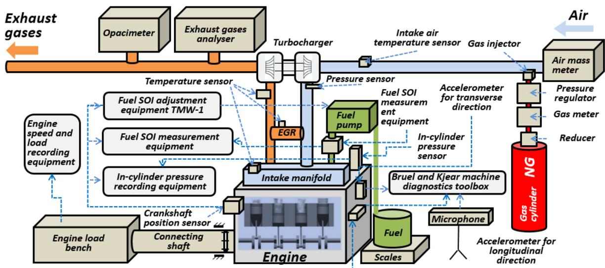
Fig. 1. Schematic diagram of experimental equipment
