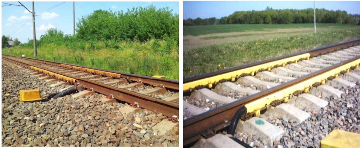
Fig. 1. System ATLAS-LG used to measure wheel-rail interaction forces
