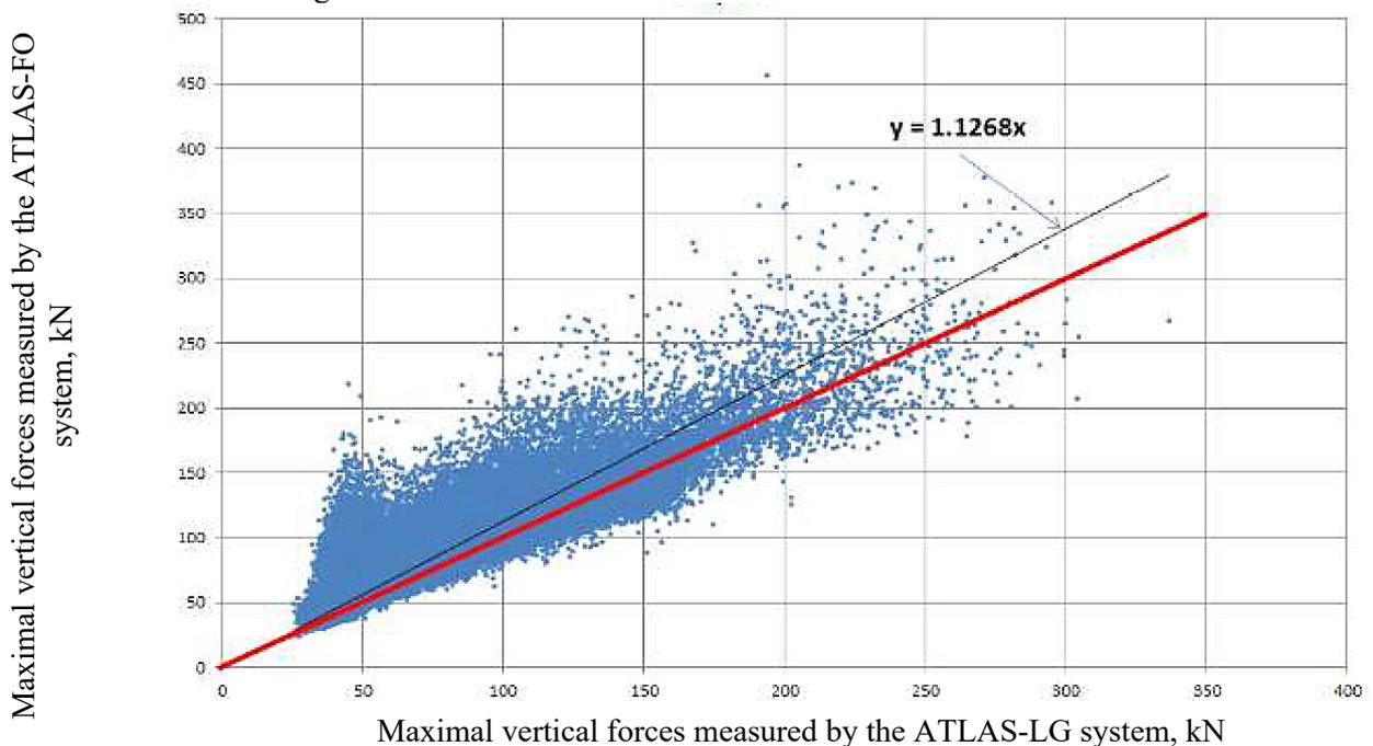
Fig. 6. The correlation comparison of maximal vertical forces measured by ATLAS-LG and ATLAS-FO in summer ( $R^2=0.886$ )
