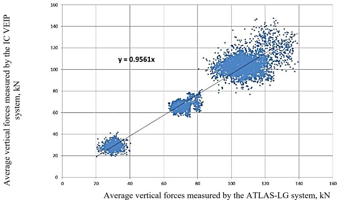
Fig. 3. Correlation comparison of average vertical forces measured by the ATLAS-LG and by IC VEIP systems ( $R^2=0.963$ )
