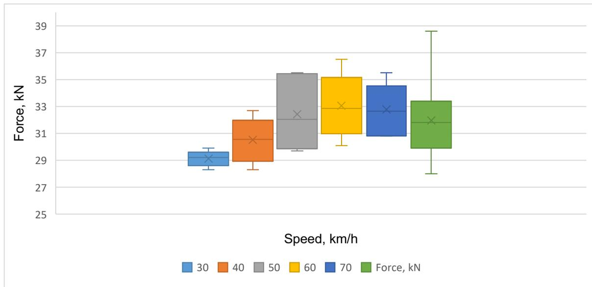
Fig. 12. Average values of vertical force when the wagon is empty
