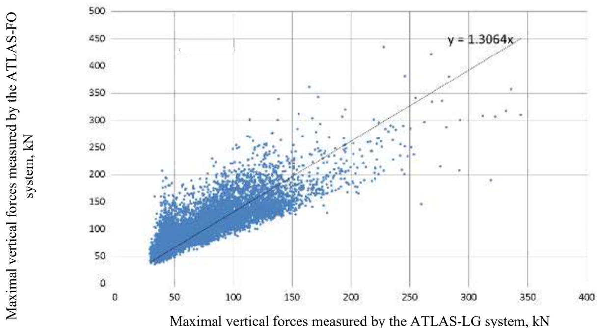
Fig. 8. Correlation comparison of maximal vertical forces measured by ATLAS-LG and ATLAS-FO in winter ( $R^2=0.848$ )
