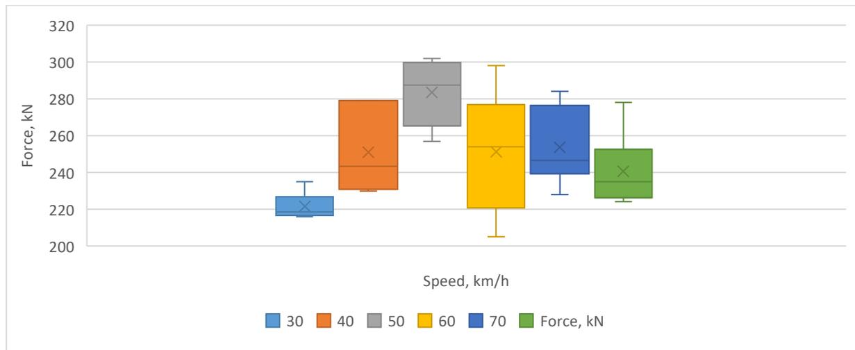
Fig. 9. Values of maximal forces when the wagon is loaded
