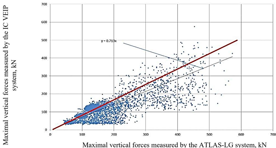
Fig. 4. The correlation comparison of maximal vertical forces measured by the ATLAS-LG and by IC VEIP systems ( $R^2=0.757$ )
