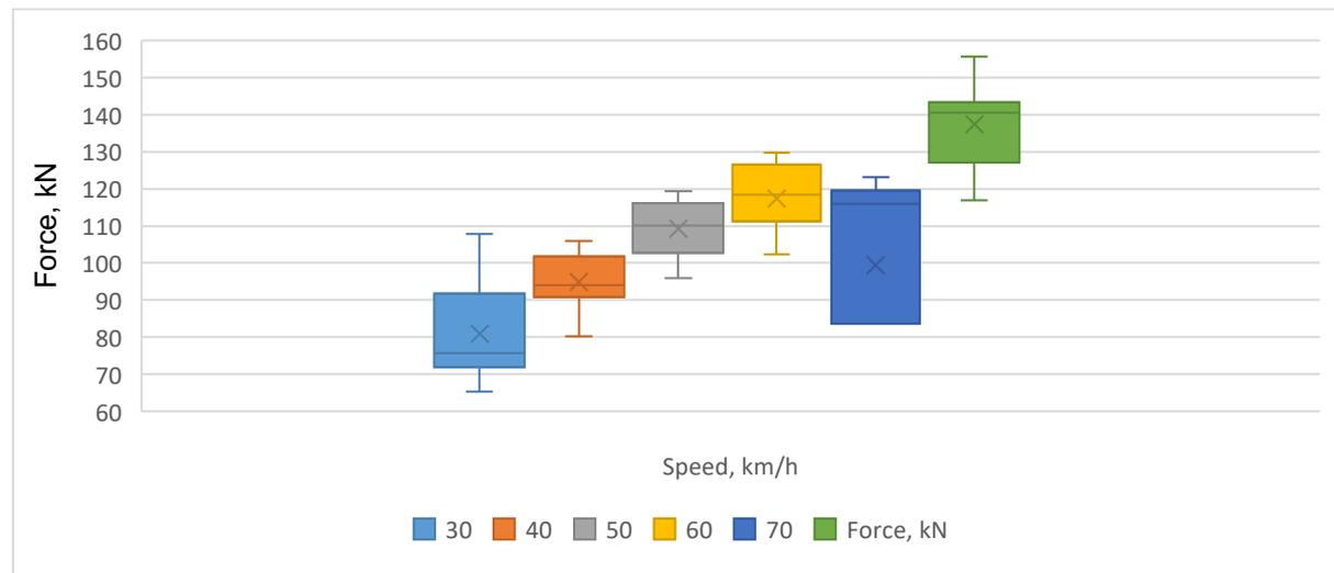
Fig. 10. Values of maximal forces when the wagon is empty
