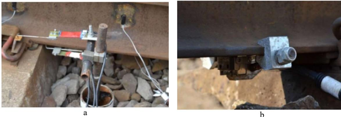
Fig. 2. Automatic rolling stock wheel damage detection systems: a) an IC-VEIP system and b) an ATLAS-FO system
