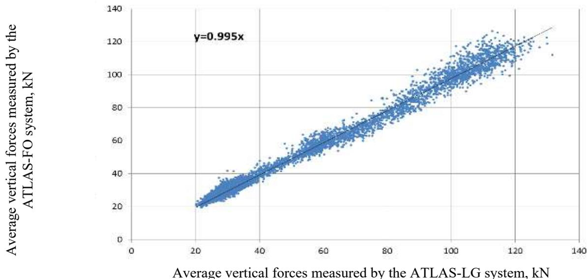
Fig. 7. Correlation comparison of average vertical forces measured by ATLAS-LG and by ATLAS-FO in winter ( $R^2=0.995$ )
