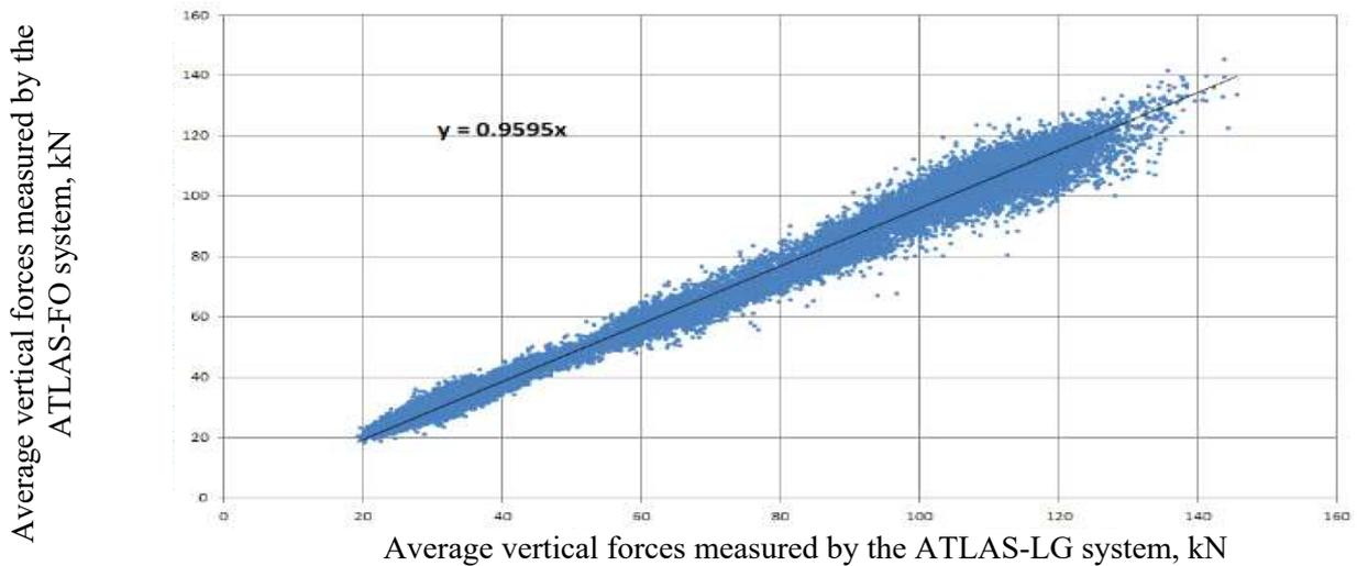
Fig. 5. Correlation comparison of average vertical forces measured by ATLAS-LG and by ATLAS-FO in summer ( $R^2=0.995$ )
