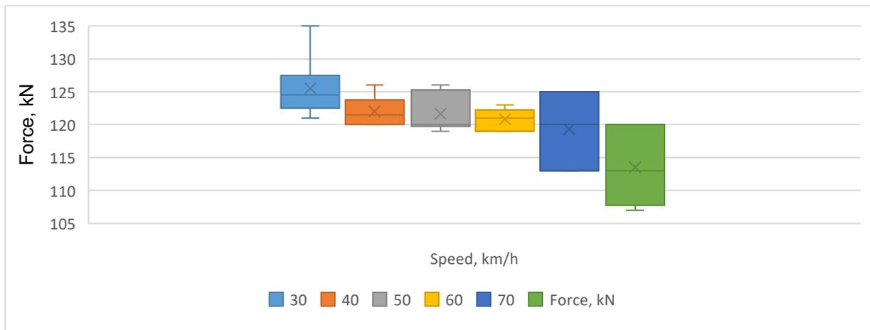
Fig. 11. Average values of vertical force when the wagon is loaded
