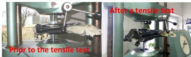
Fig. 10. Specimen no. 1 in the holder of the universal testing machine prior to and after the specimen broke apart
