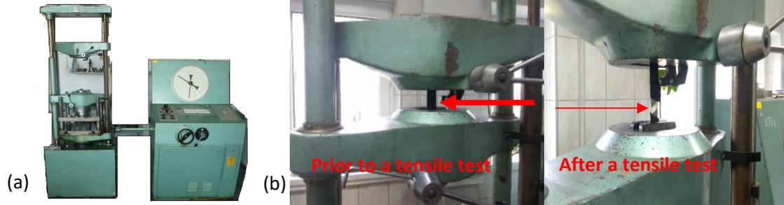
Fig. 5. Photographs of (a) the strength testing stand (ZD-20) and (b) specimen no. 1 mounted in the jaws of the testing machine prior to and after the tensile test
