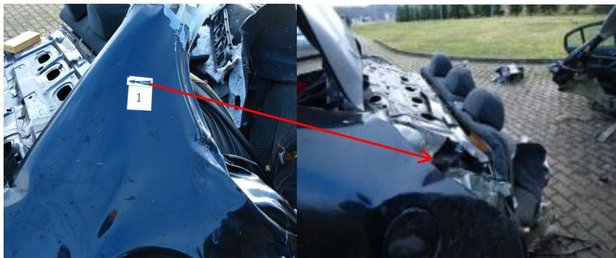
Fig. 3. View of the place of the specimen taken from the Škoda body
