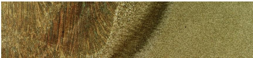
Fig. 4b. Macrograph of the weld (S2) with clearly marked HAZ (in the middle of the photo)
