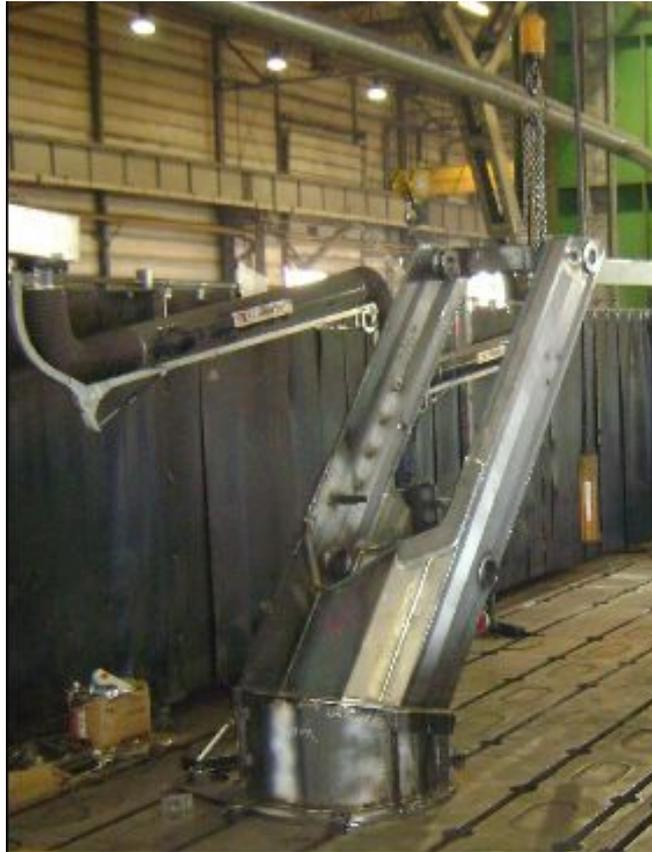
Fig. 7. A mobile platform arm welded using the newly obtained technology
