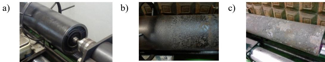
Fig. 4. Type C roll tested before assembly (a), C type roll disassembled after 12 months of operation (b), and 24 months of operation (c) from conveyor
