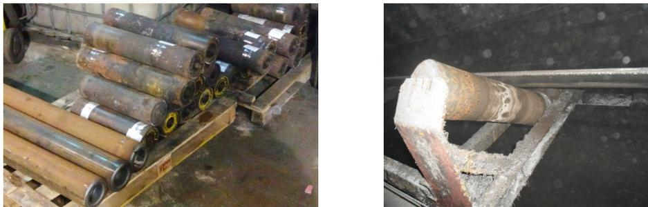
Fig. 1. Rollers selected for testing disassembled from a belt conveyor in a coal mine
