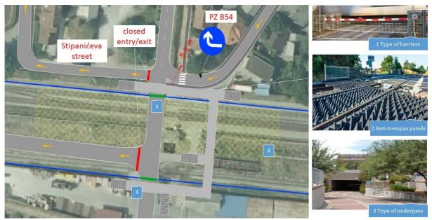
Alternative 1 considers the construction of a pedestrian and cyclist underpass (Fig. 5).
