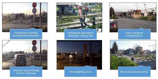
Fig. 2. Problems at LC Sokolska (poor infrastructure and level crossing users' behaviours)
