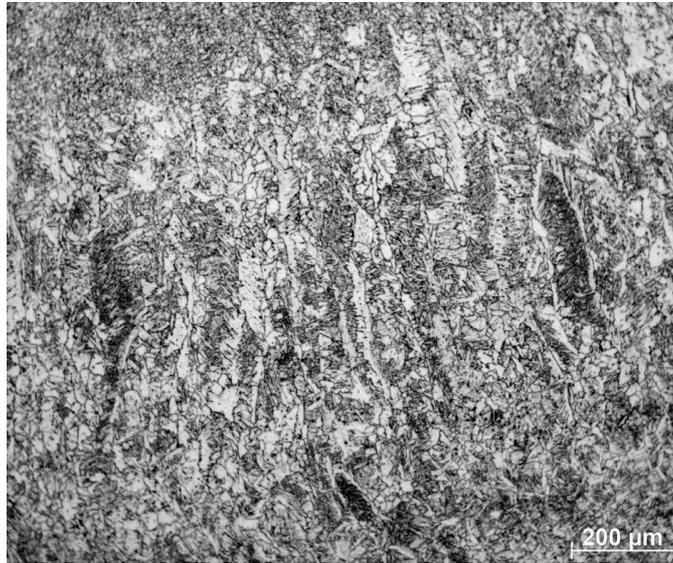
Fig. 3. Acicular ferrite in S235JR weld (60%) after He micro-jet cooling
