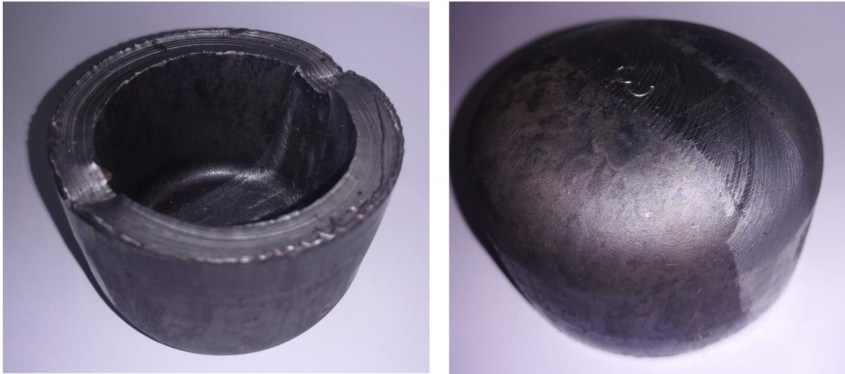
Fig. 5. One of the obtained cylindrical vessels from the inside and outside. Stamping of weld with MJC
