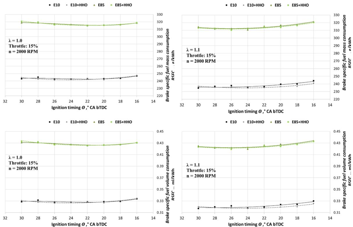
Fig. 4. Brake-specific fuel mass and volume consumption
