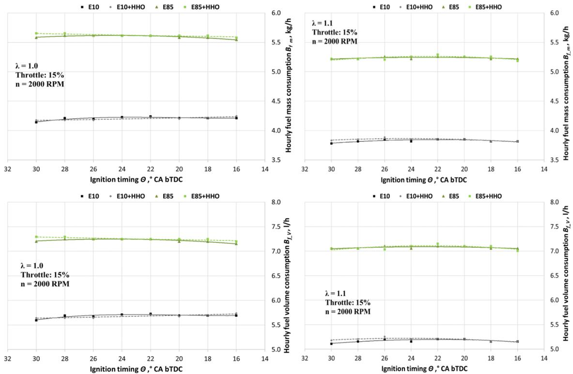
Fig. 3. Hourly fuel mass and volume consumption
