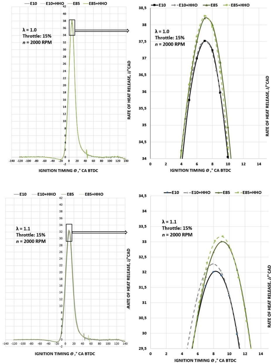
Fig. 6. Rate of heat release
