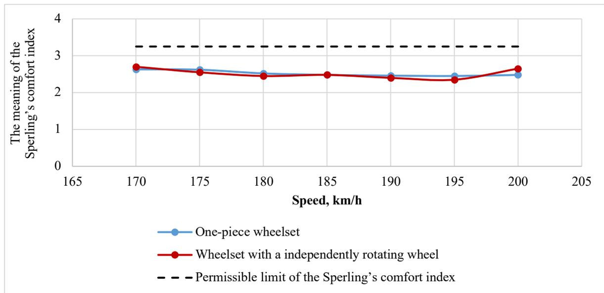
Fig. 9. Sperling's comfort index values in the vertical direction in the 2900 m radius curve
