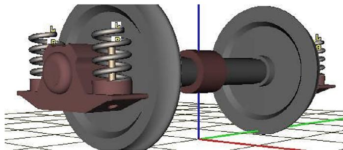
Fig. 2. Wheelset with independently rotating wheels
