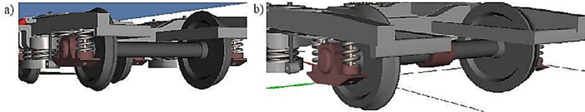
Fig. 4. Bogie model of passenger cars in “Universal Mechanism” software: a) with integral wheelsets and b) with independently rotating wheels
