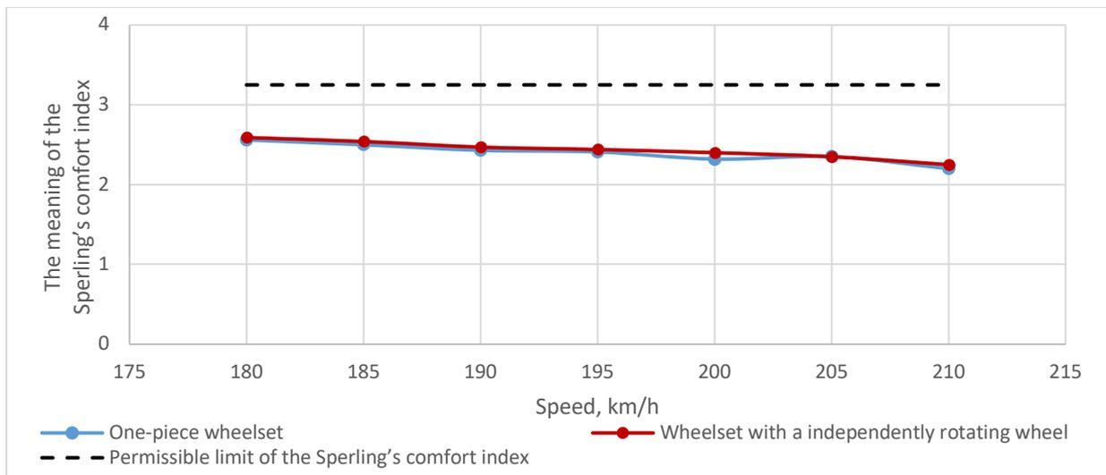
Fig. 11. Sperling's comfort index values in the vertical direction in the straight section
