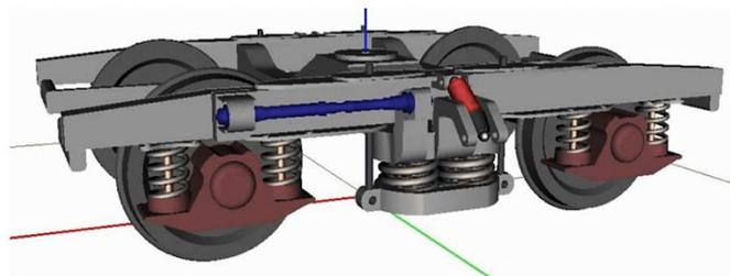
Fig. 3. Structure of a passenger car bogie
