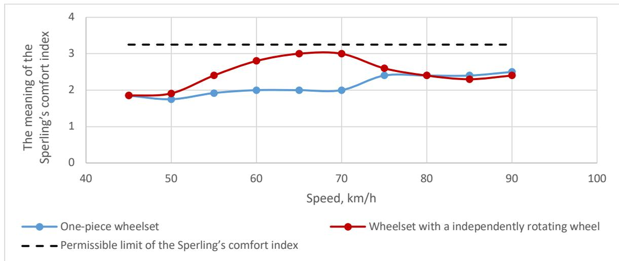
Fig. 8. Sperling's comfort index values in the lateral direction in the 200 m radius curve
