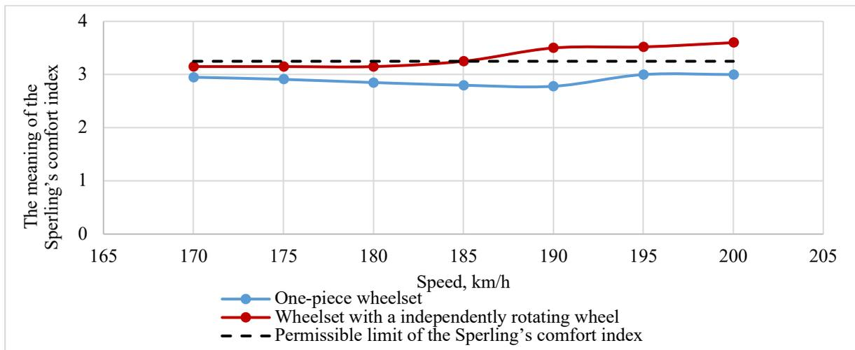
Fig. 10. Sperling's comfort index values in the lateral direction in the 2900 m radius curve
