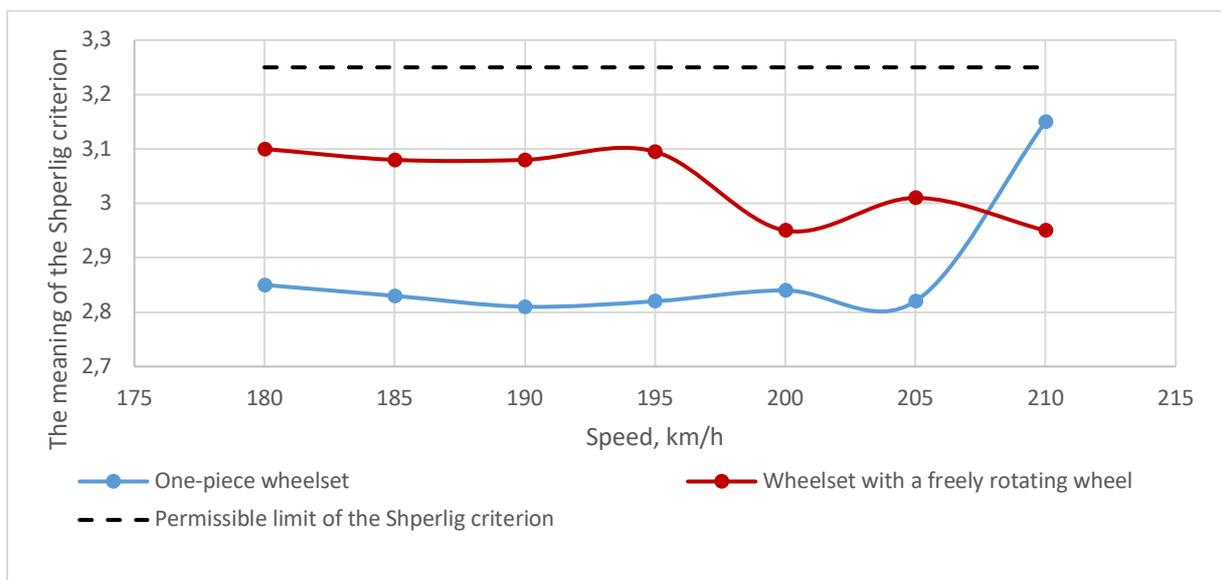
Fig. 12. Sperling's comfort index values in the lateral direction in the straight section
