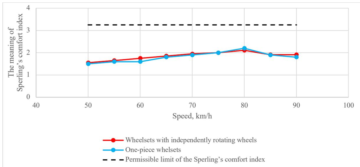
Fig. 7. Sperling's comfort index values in the vertical direction in the 200 m radius curve
