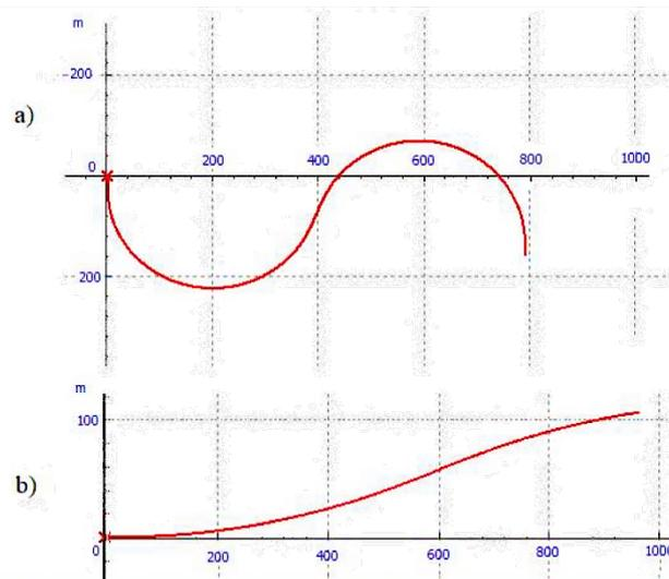
Fig. 6. Track curve geometries of the modeled S type: a) when  $R = 200$  m and b) when  $R = 2900$  m
