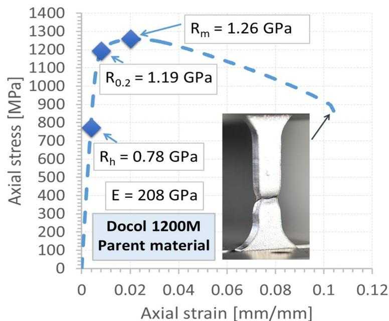
Fig. 4. Tensile characteristic with mechanical parameters and its fracture zone of the Docol 1200M,  $R_m/R_{0.2} = 1.05$ , where: E – Young modulus,  $R_h$  – Hook limit,  $R_{0.2}$  – conventional yield point,  $R_m$  – ultimate tensile strength
