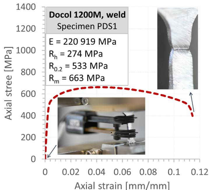
Fig. 6. Tensile characteristic and mechanical parameters of the weld to Docol 1200M  $R_m/R_{0.2} = 1.24$
