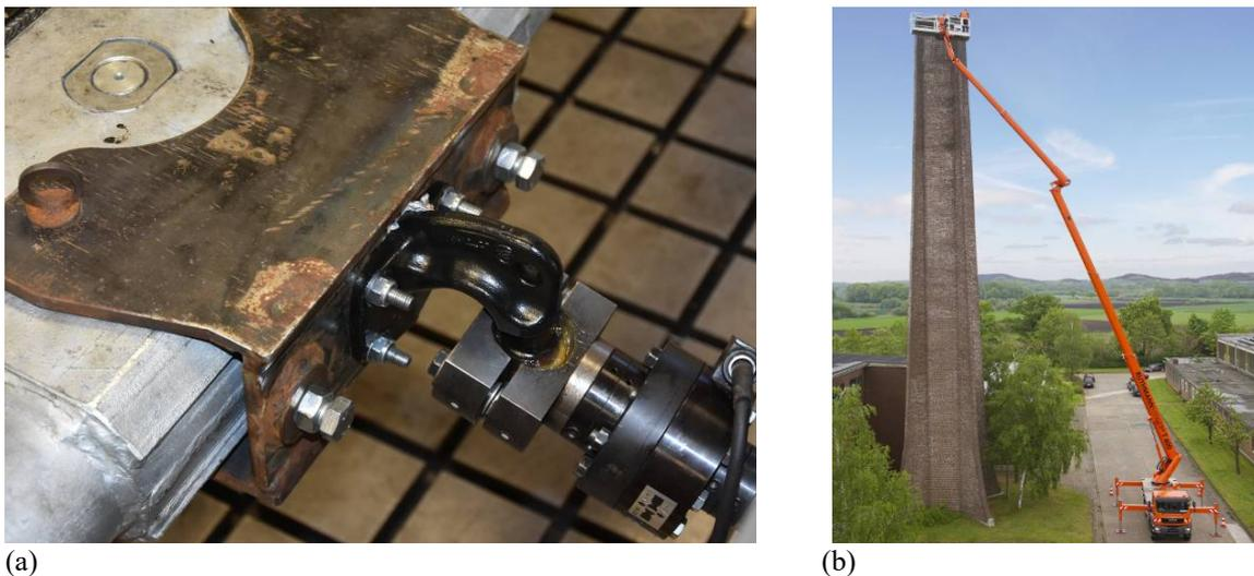
Fig. 1. Application of advanced high-strength steel: (a) a region of towing boom used for coupling vehicles, (b) mobile platform on a special vehicle [12]
