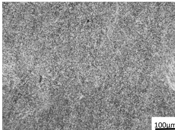
Fig. 9. Structure of the cross-section MAG weld with the use of m-j cooling
