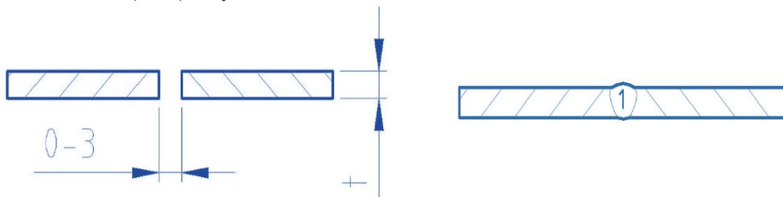
Fig. 5. Details for preparation of the elements for MAG welding with micro-jet (m-j) cooling, thickness  $t = 3$  mm
