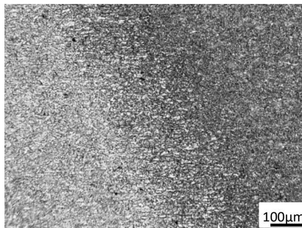
Fig. 10. Structure of the fusion line. On the left is presented base material, on the right HAZ
