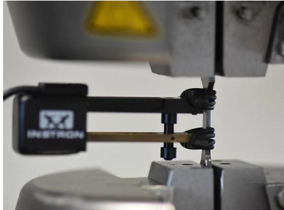
Fig. 3. Flat specimen with extensometer before tensile test
