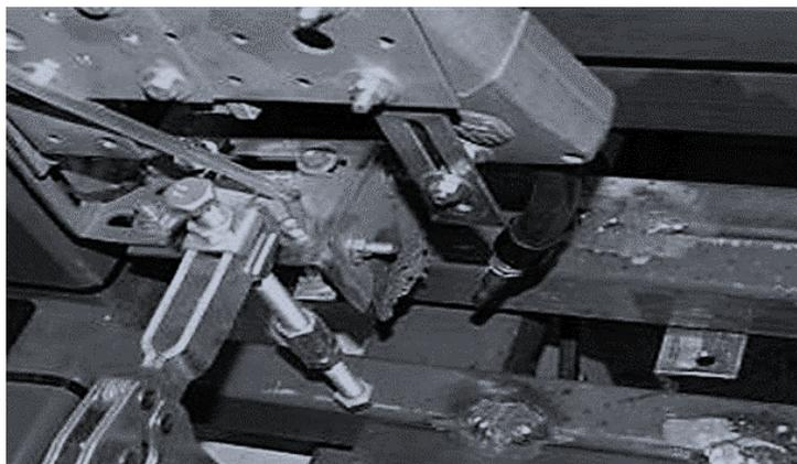
Fig. 2. Welding station with cooling injector
