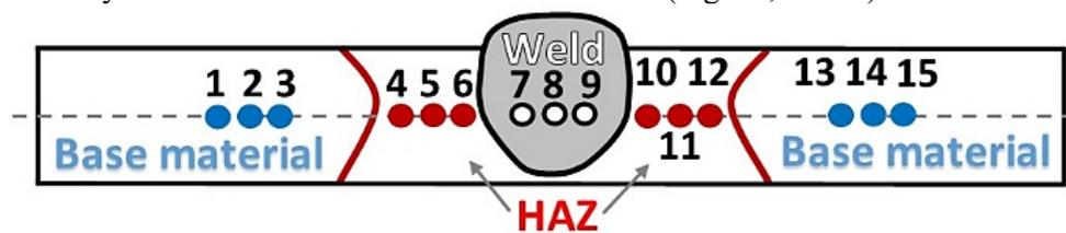
Fig. 11. A scheme of the hardness measurements for the welded joint manufactured at the micro-jet cooling
