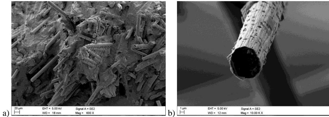
Fig. 6. Polymer composite on a polyamide matrix: a) single carbon fibre with TiN layer deposited on the outside, b) [the authors own work]
