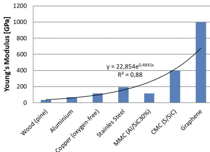
Fig. 19. Comparison of Young's modulus of basic construction materials used for aircraft construction based on [27-29]
