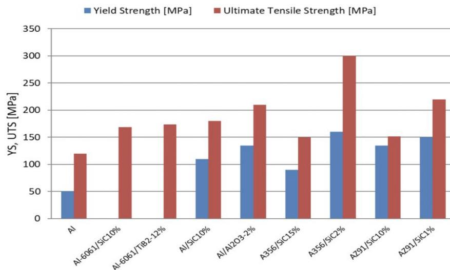
Fig. 5. Impact of the reinforcement type on the strength properties of composites; Al-6061/SiC12% reinforcement particle size 40-45µm; Al-6061 / TiB<sub>2</sub>-10% - 1-2 µm; Al/SiC10% - 10µm; Al/Al<sub>2</sub>O<sub>3</sub> 2% - 25 nm; A356 / SiC15% - 40 µm; A356/SiC2% - 20-30 nm; AZ91/SiC10% - 7µm; AZ91/SiC1% - 30 nm [12]
