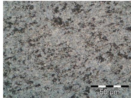
Fig. 3. Ceramic Matrix Composite F1200, with aluminium oxide matrix reinforced  $B_4C$  [the authors own work]
