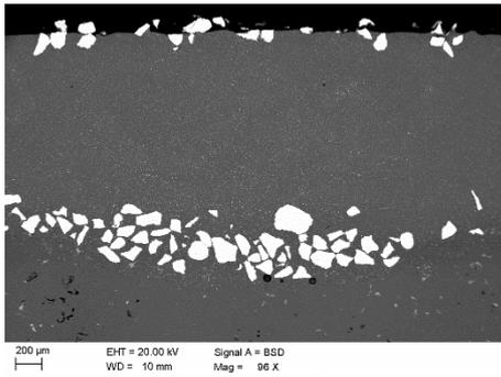
Fig. 11. The surface layer of AlSi9Cu alloy after melting the ceramic powder, laser power 2.0 kW, 1.5 g/min, remelting rate 0.25 m/min
