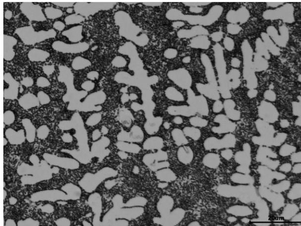
Fig. 9. The structure of aluminum alloy 6082 weld made with MIG method
