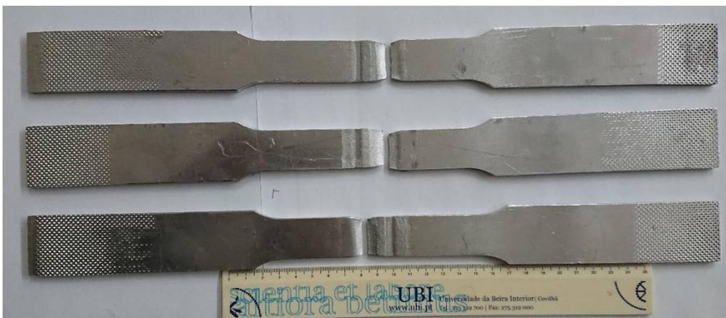
Fig. 8. Samples from alloy 6082 after rupture
