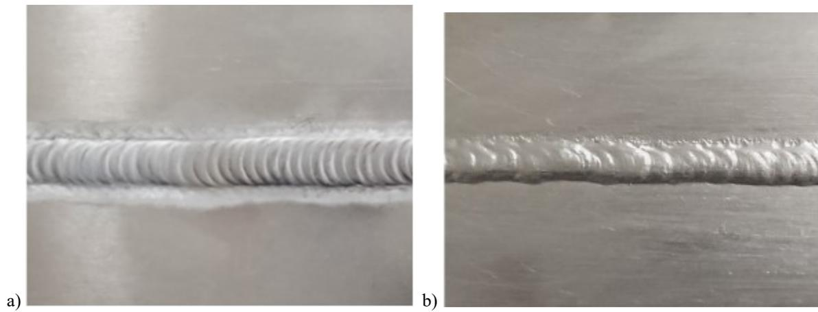
Fig. 6. Samples from 6082 aluminum alloy welded with different methods: a) TIG; b) MIG
