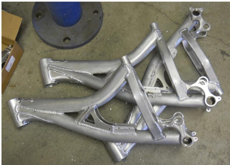
Fig. 3. Frame welded with the MIG method [13]
