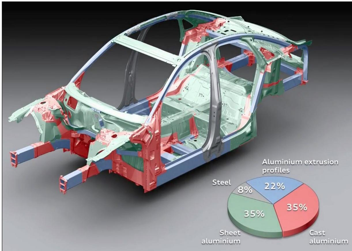
Fig. 1. Aluminum frame in self-supporting car -body structure [11]
