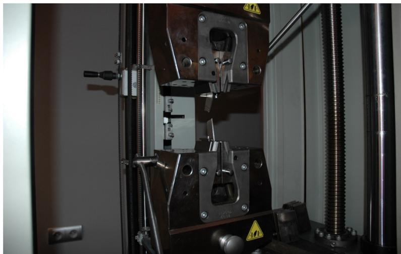
Fig. 7. Tensile test carried out on a ZWICK 100N5A type machine
