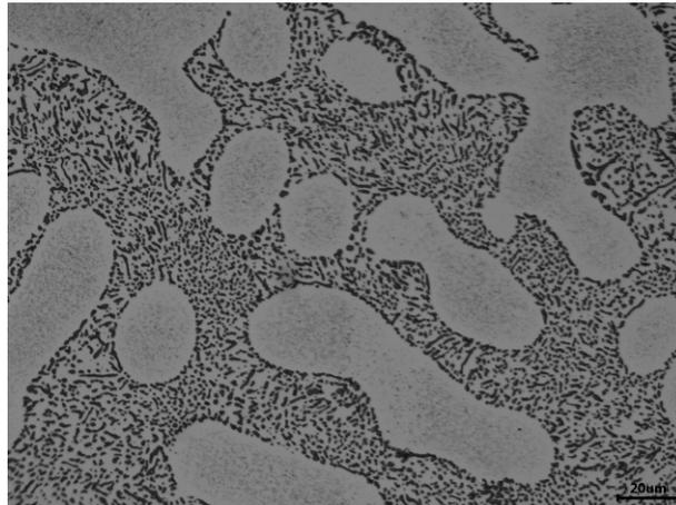
Fig. 5. The structure of 6082 aluminum alloy in delivery condition
