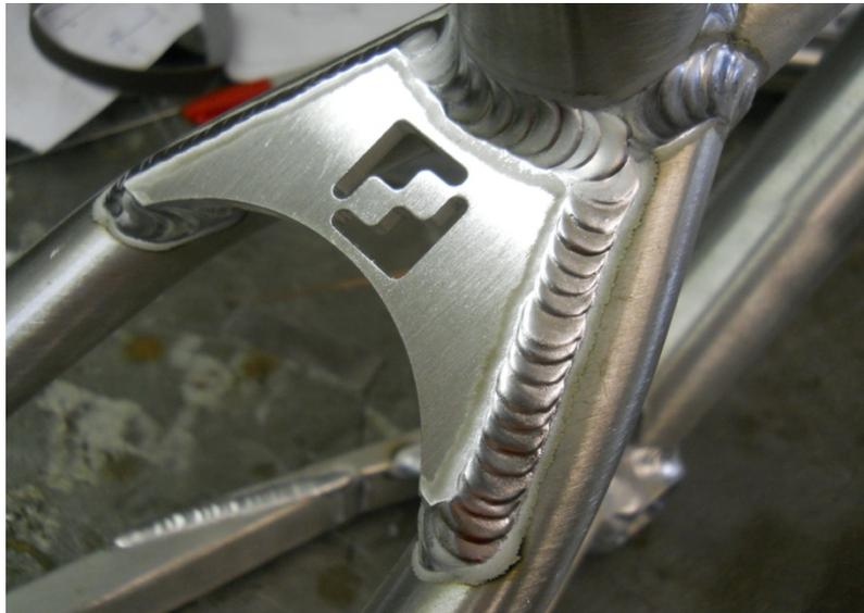
Fig. 2. Frame welded with the TIG method [12]
