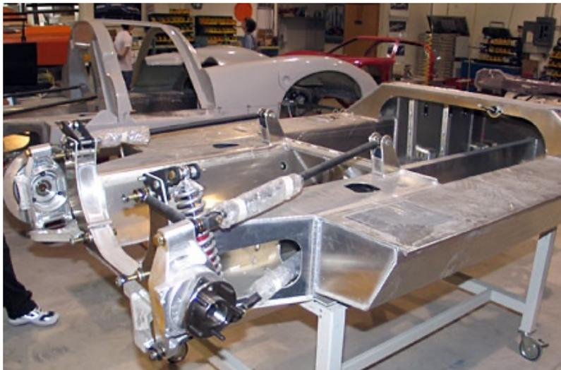
Fig. 4. Frame structure welded with the TIG method [13]
