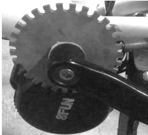
Fig. 4. Unique incremental encoder combining a toothed metal disk and an optical sensor
