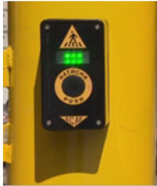
Fig. 1. Button of a traffic light for alerting the system a pedestrian is waiting
