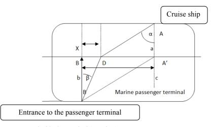
Fig. 3. Moving passengers inside the terminal (top view)
