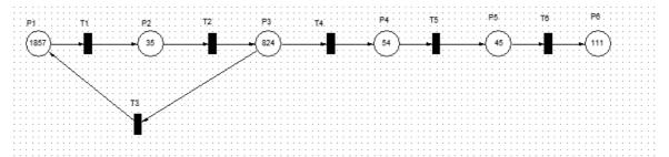
Fig. 5. Petri net model of logistical chain of movement of passengers in the port
