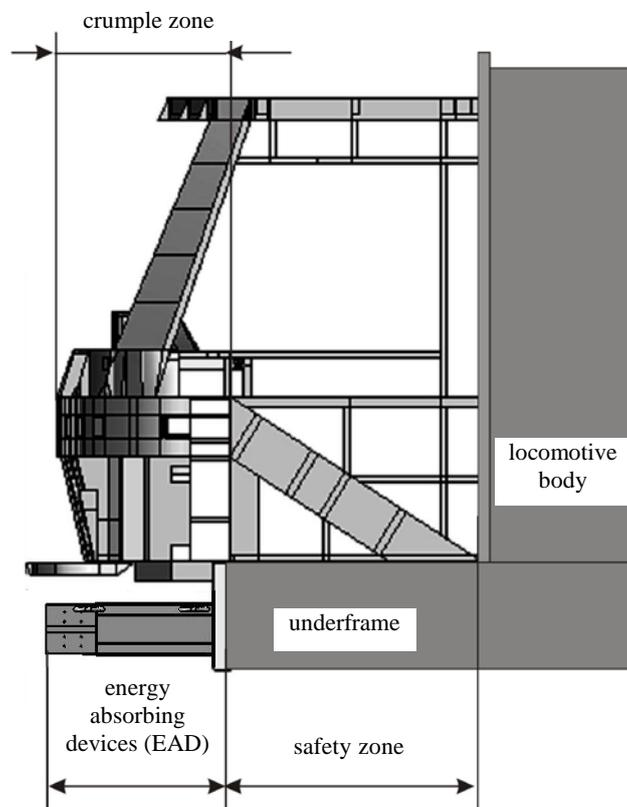
Fig. 2. Design layout scheme of the driver's cab frame with energy-absorbing devices
