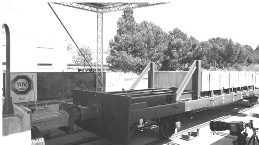
Fig. 6. Crash test of the energy-absorbing device prototype
