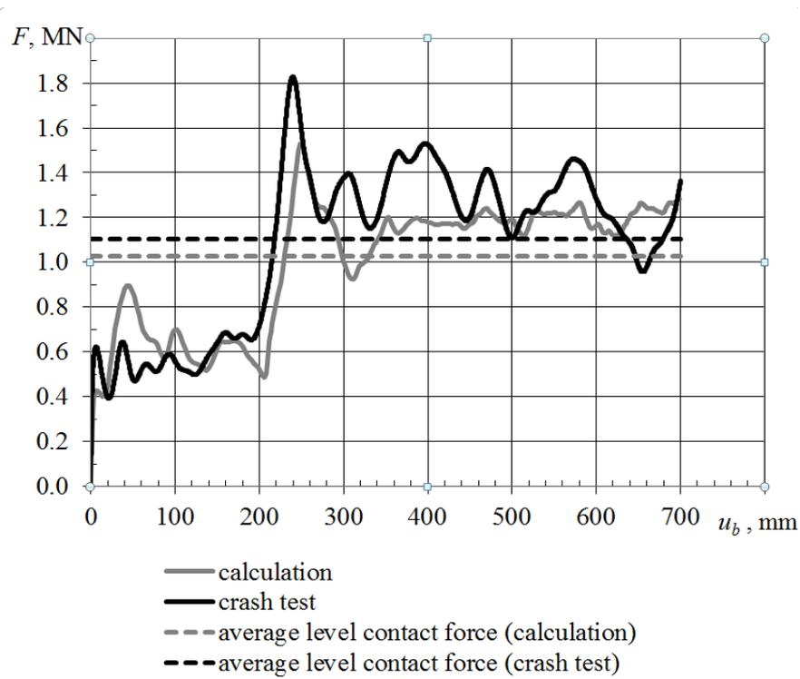
Fig. 9. The calculated and experimental dependencies of a contact force  $F$  on the displacement  $u_b$
