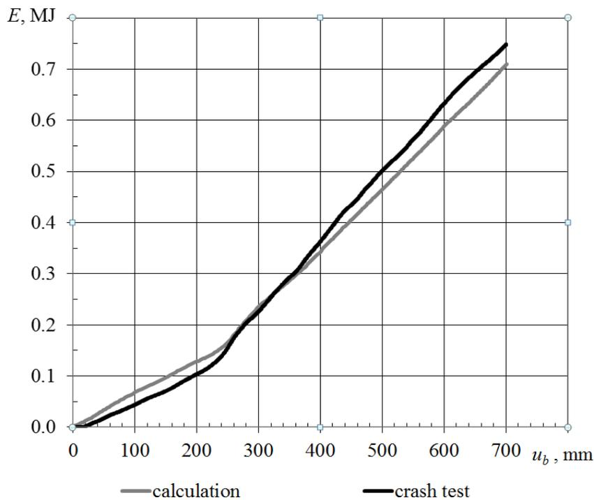
Fig. 10. The calculated and experimental dependencies of an absorbed energy  $E$  on the displacement  $u_b$
