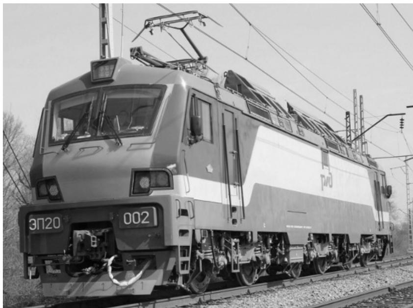
Fig. 1. High-speed passenger electric locomotive EP20
