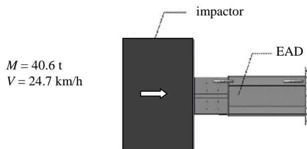
Fig. 7. The scheme of interaction between the EAD and the wagon-impactor
