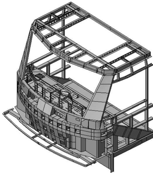
Fig. 3. The driver's frame cab design for the locomotive with a passive safety system
