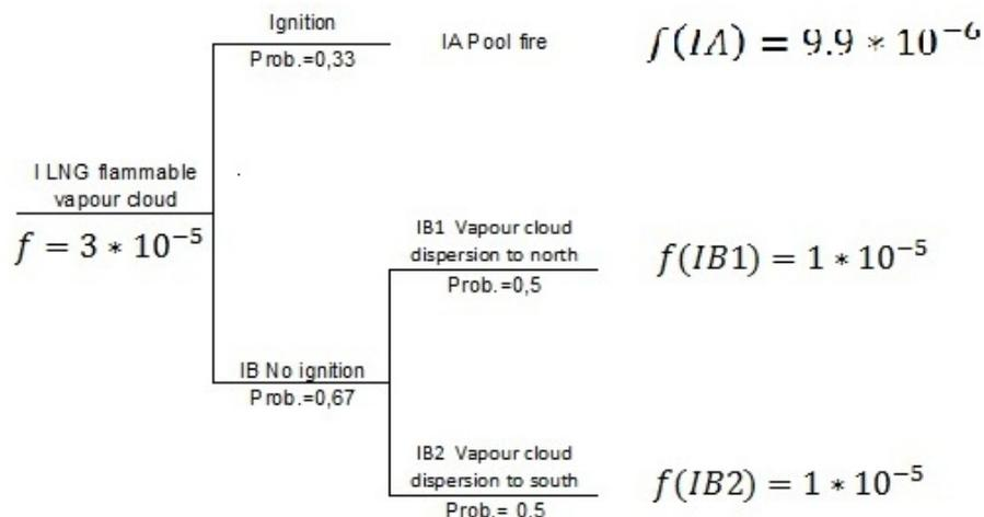
Fig. 6. Frequency estimates for the example incident
