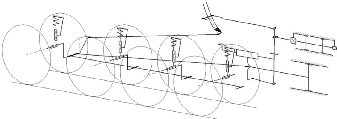
Fig. 3. Half model of the steam locomotive's Gr-319 running gear and piston engine, valve gear (for clarity, all wheels are shown)
