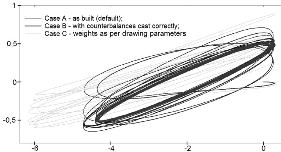
Fig. 6. Locomotive's centre of gravity trajectory along x and y axis, mm (start of calculations – point 0, 0)
