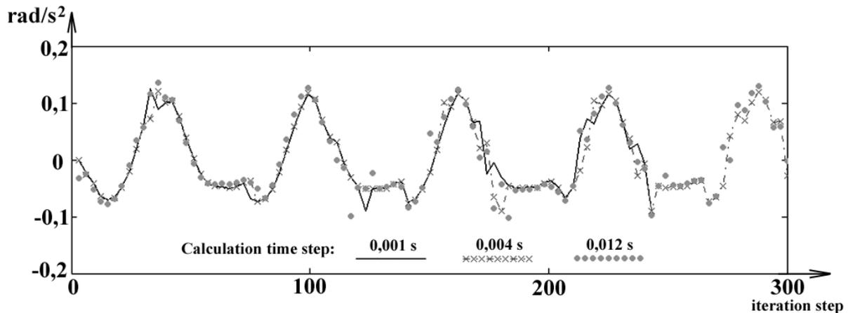
Fig. 5. Angular acceleration of the locomotive upper structure (roll vibrations),  $\text{rad/s}^2$
