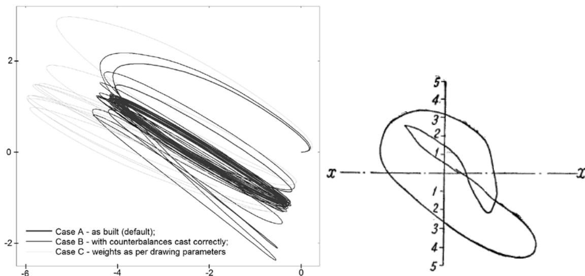
Fig. 4. Left – calculated trajectory of the driver's seat along x and y axis (mm), right – for comparison data from locomotive E Nr. 5570, as given in [5]
