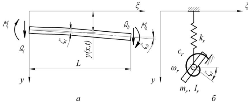
Fig. 3. Diagram of monorail strain: *a* – *s* segment; *b* – support fastening assembly
