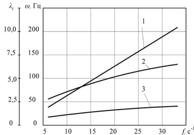
Fig. 4. Dependences: 1 –  $\omega(f)$ ; 2 –  $\lambda_1(f)$  if  $L_1=6$  m; 3 –  $\lambda_2(f)$  and  $L_2=3$  m
