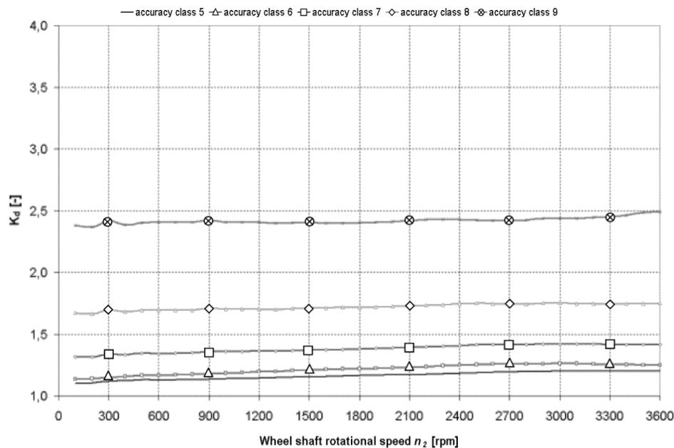
Fig. 5. The relationship of the dynamic load coefficient  $K_d$  on the rotational speed  $n_2$  of the shaft of a wheel and on the accuracy class (according to Maag modified spur gears, unit load  $Q = 2$  MPa)
