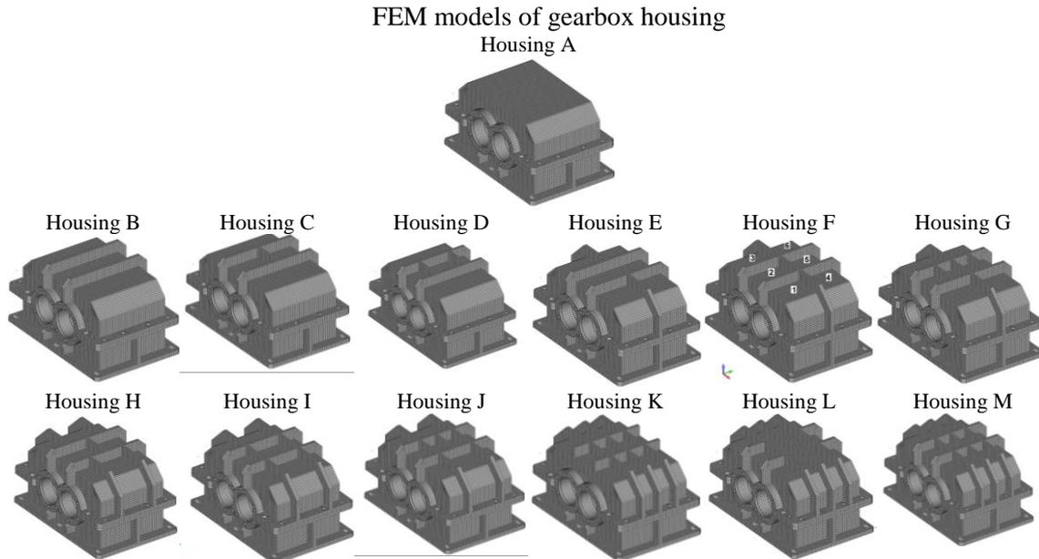
In order to further verify the tuned FEM models of the gearbox housing, stand tests and numerical tests were performed which resulted in determining the values of normal vibration velocity in six selected measuring points on the upper cover of the gearbox housing. The compatibility of results of the active and numerical experiments made for three designs of gearbox housings enabled confirming the correctness of the FEM models elaborated.
