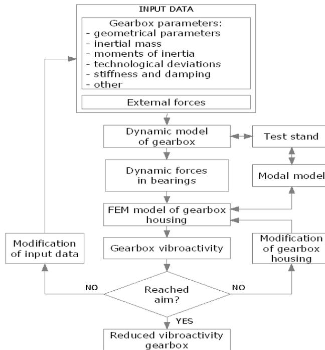
Fig. 1. Design methodology for gearboxes with reduced vibroactivity
