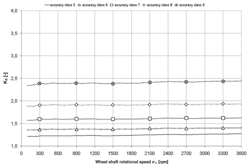
Fig. 7. The relationship of the dynamic load coefficient  $K_d$  on the rotational speed  $n_2$  of the shaft of a wheel and on the accuracy class (spur gears with negative value of the profile deviation,  $Q = 3$  MPa)
