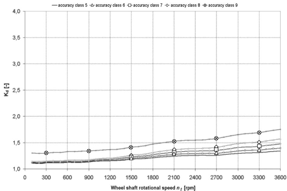
Fig. 6. The relationship of the dynamic load coefficient  $K_d$  on the rotational speed  $n_2$  of the shaft of a wheel and on the accuracy class (spur gears with positive value of the profile deviation,  $Q = 3$  MPa)
