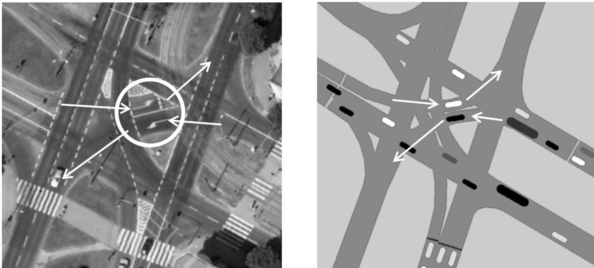
Fig. 2. Intersection 5 – an aerial photography and the model in VISSIM
