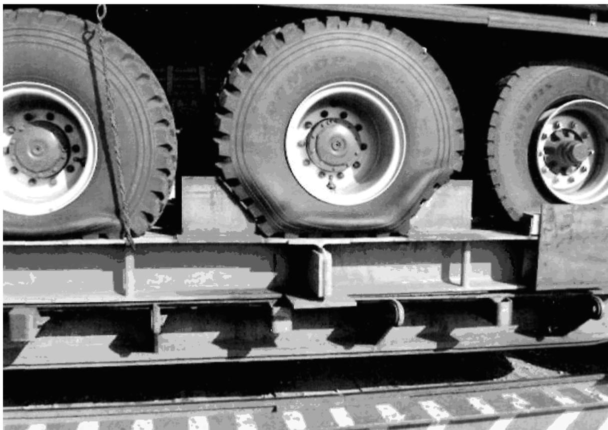
Fig. 3. Pressure reduction of wheel machinery wheels on a flat car
