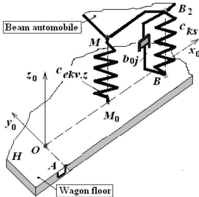
Fig. 7. Intermediate model of wheel machinery allocated on a flat car
