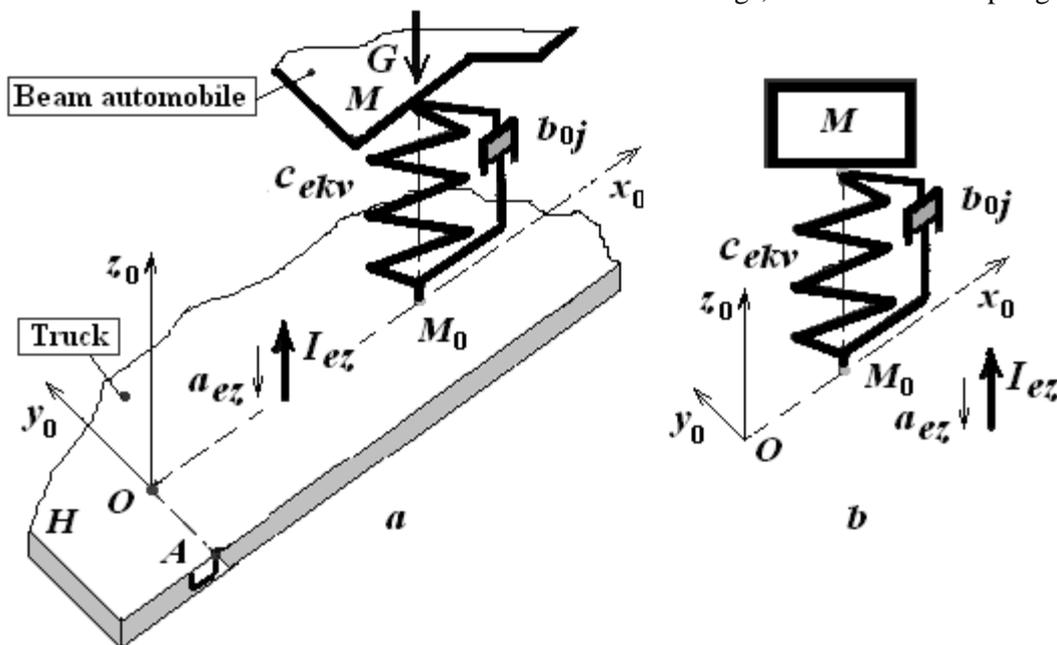
Fig. 8. Dynamical modeling of wheel machinery: *a* – WM body, connected with flat car by elastic element and viscous environment; *b* – single-mass WM model on vibrating base
