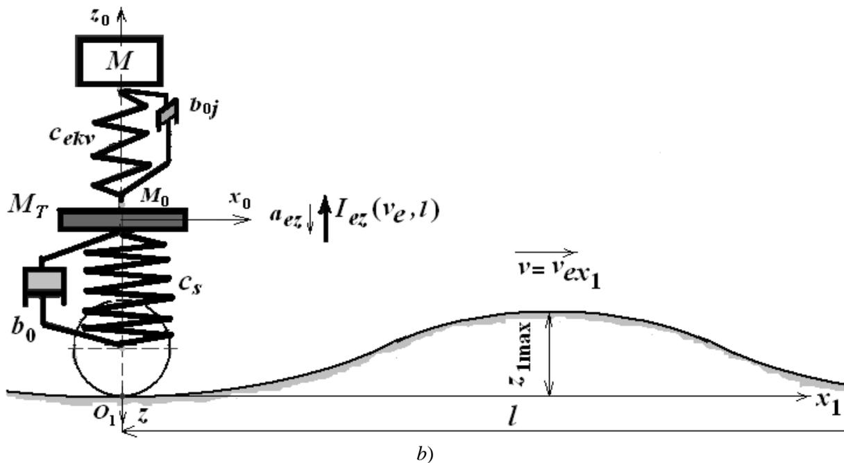
Fig. 9. Mechanical system “single-axe vehicle – flat car – wheel machinery” *a)* –dynamical modeling of wheel machinery and flat-car as single-axe vehicle with dry friction force; *b)* – two-mass vibrating system with elastic elements and viscous media
