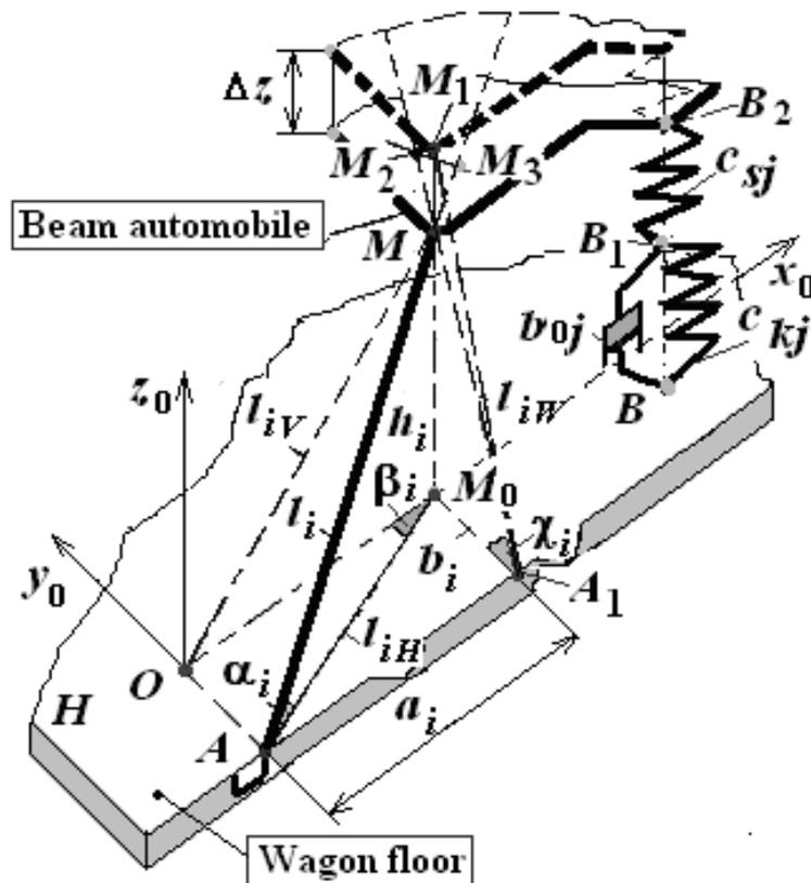
Fig. 5. Lengthening of fastening elastic element relative to vertical
