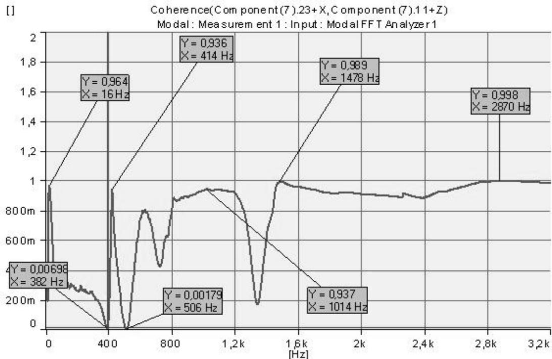
Fig. 4. The diagram of coherence using modal FFT analyser
