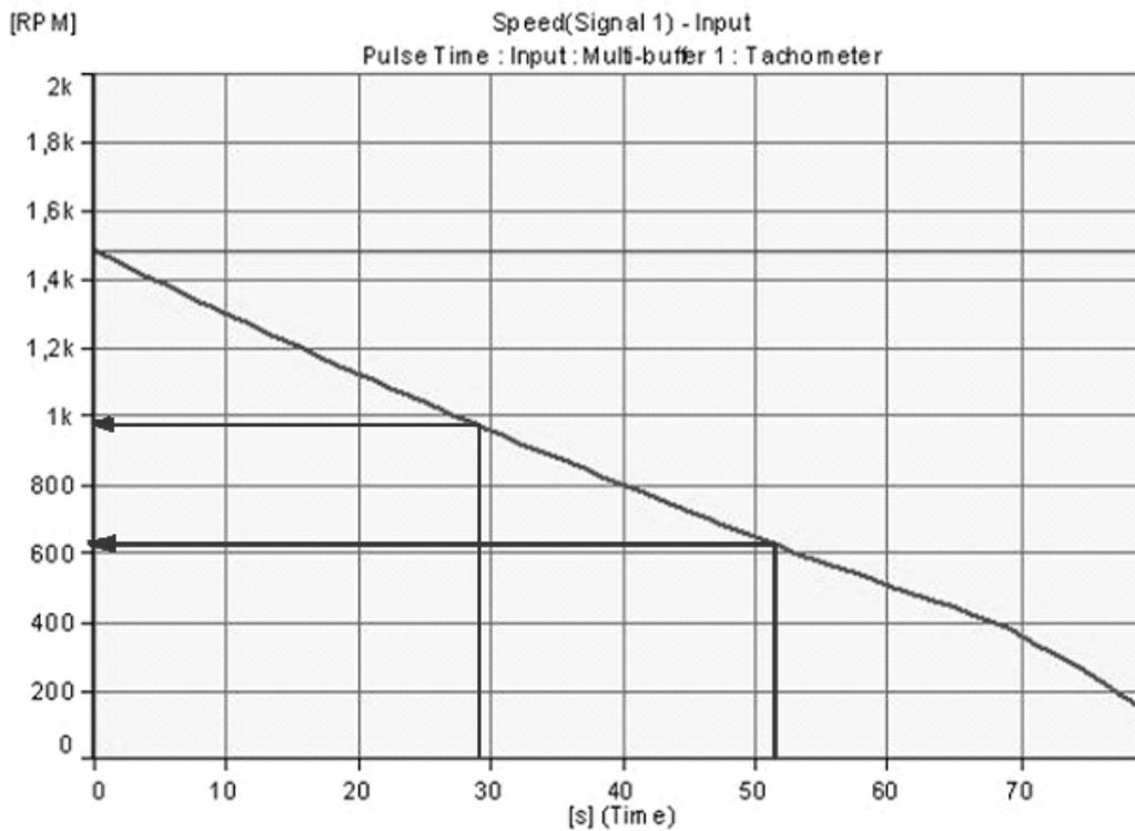
Fig. 11. Characteristic of rotors rotational speed during free stop-down deceleration
