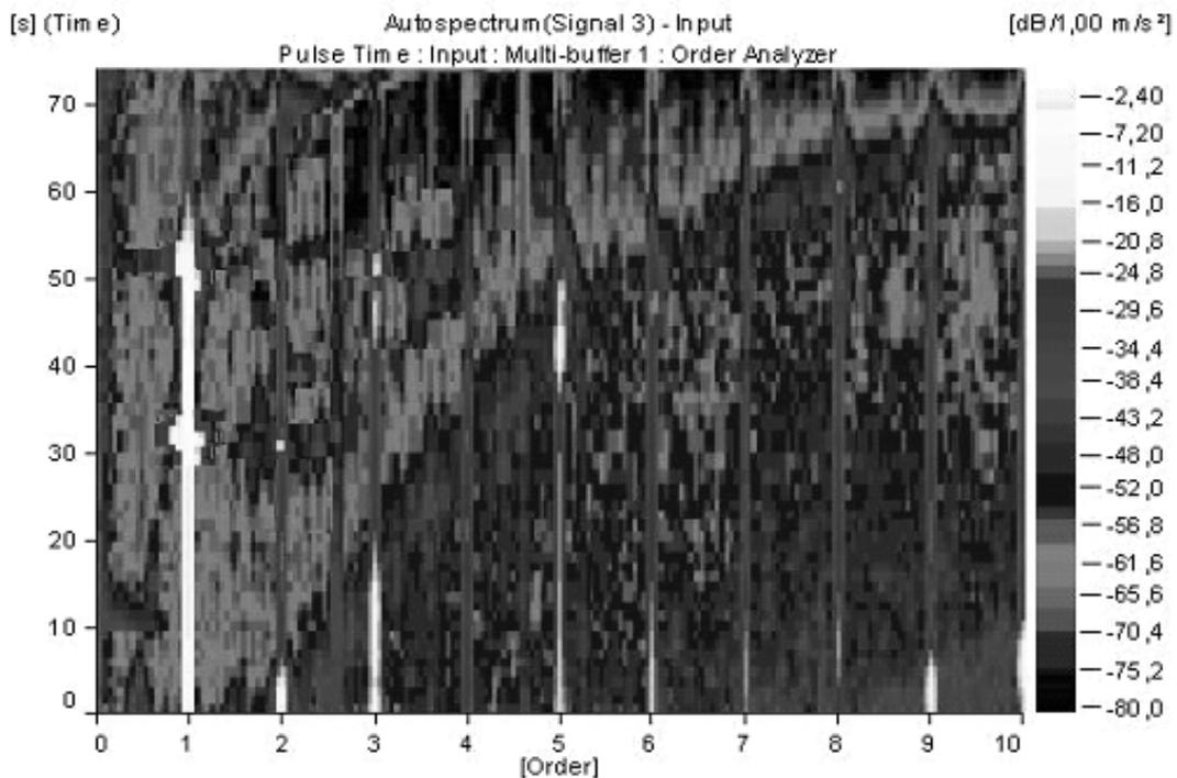
Fig. 10. Order tracking procedure for free stop-down process of the rotor
