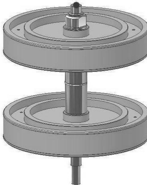
Fig. 8. Second stickseed support of rotor
