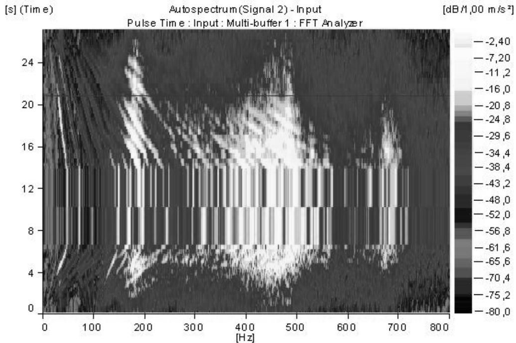
Fig. 9. Autospectrum FFT of acceleration with forced breaking of rotor
