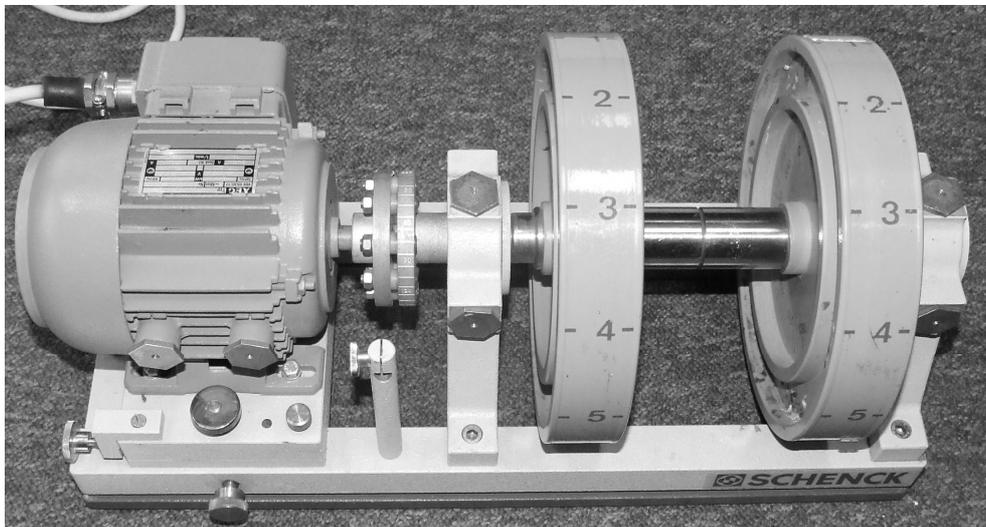
Fig. 1. Simplified laboratory model of gas turbine rotor
