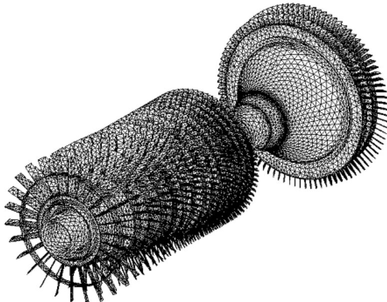
Fig. 5. Virtual model of LM 2500 gas generator
