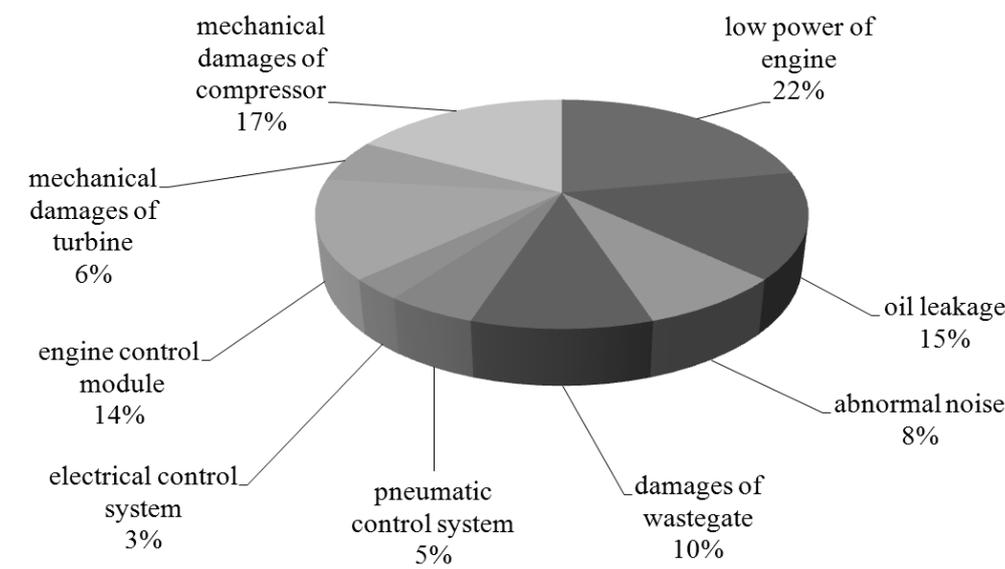
Fig. 4. Structure of engine faults connected with turbocharger
