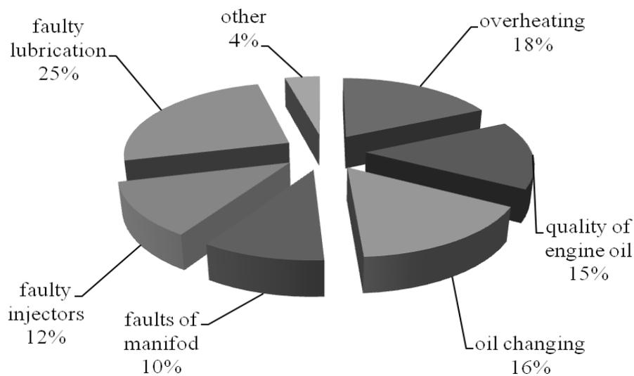
Fig. 5. Structure of causes of turbocharger faults
