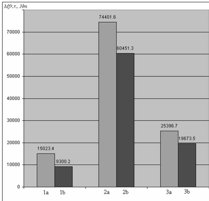
Fig. 5. Values of  $M_{fr.r.}$  calculated according to (4) for three states of leaning of basket of freight carriage: a) in the case of absence of greasing and b) at presence of greasing: 1 is the frame with the load leaning only against the center plate of the train beam, 2 is the frame with the load leaning against the center plate and one of the slide-block; 3 is the frame with the load leaning against the center plate and the skating rinks, set on the slide-block
