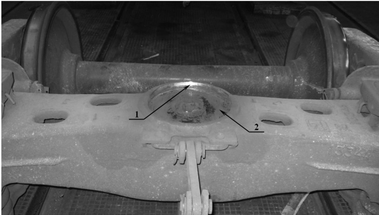
Fig. 2. Worn element of light model cart 18-100: 1 is a pad of the center plate, 2 is underlayment of the center plate
