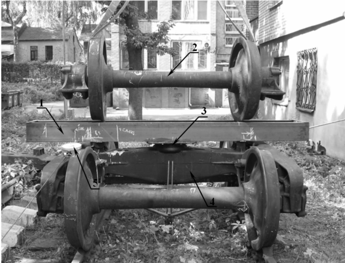
Fig. 3. Experimental system to determine the friction resistance momentum in a supporting place from forces of resistance to the rotating of the light cart. Component elements of the system: 1 is a frame, 2 is a weight, 3 is a supporting knot, 4 is a light model cart 18-100, 5 is a dynamometer and rope, related to the jack
