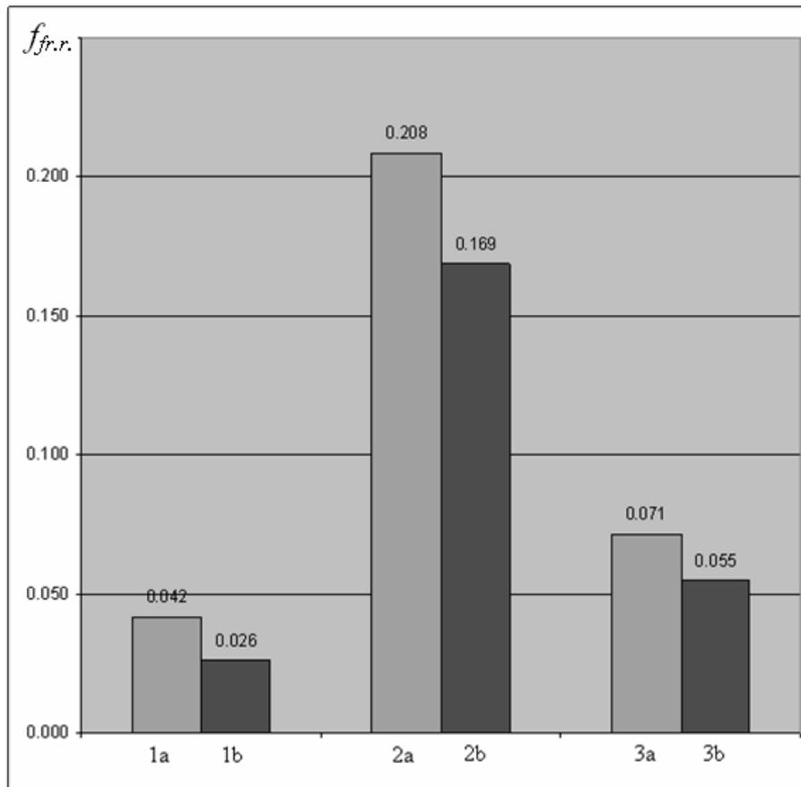
Fig. 4. Value of proportionality coefficient  $f_{fr.r.}$  calculated according to (3) for three positions of the load; a) in the case of absence of greasing; b) at presence of greasing: 1 is the frame with the load leaning only against the center plate of the train beam, 2 is the frame with the load leaning against the center plate and one of the slide-block; 3 is the frame with the load leaning against the center plate and the skating rinks, set on the slide-block
