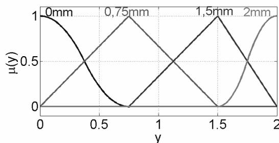
Fig. 8. Way number 2 of construction of the fuzzy outputs of the fuzzy logic system for a damage in the form of the chipping tip of the tooth
