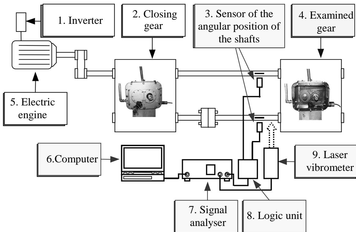
Fig. 2. Scheme for the measuring system (1-inverter, 2-closing gear, 3-sensor of the angular position of the shafts, 4- the examined gear, 5- electric engine, 6-computer, 7- the signal analyser, 8- logic unit, 9- laser vibrometer)
