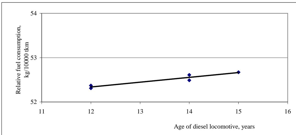
Fig. 2. Variation of fuel consumption of diesel locomotives
