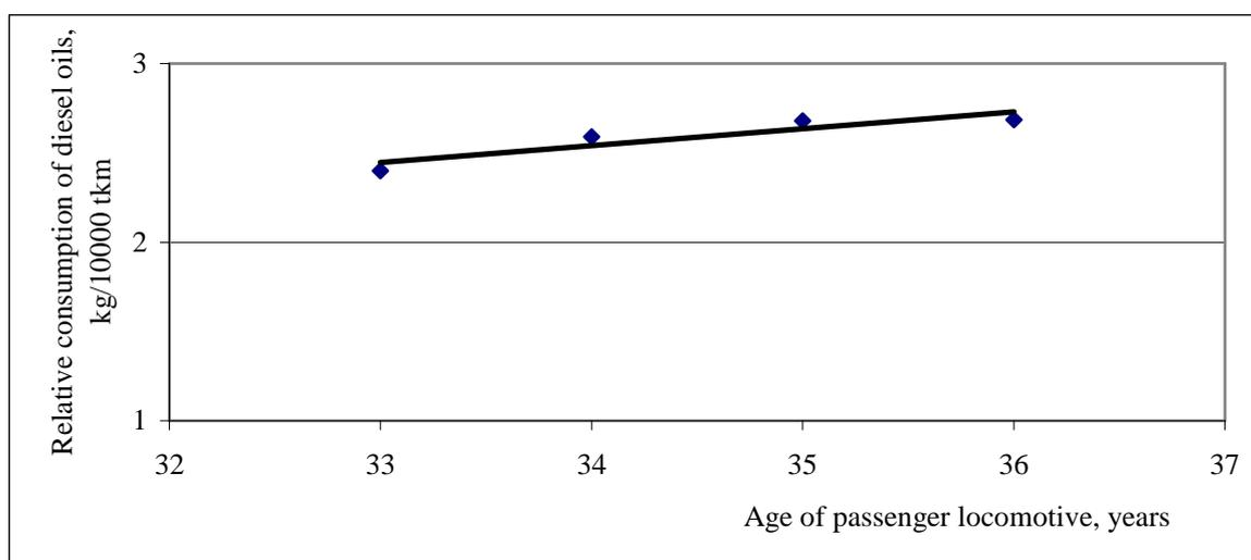
Fig. 3. The relationship between relative consumption of diesel oil by passenger locomotives and their age
