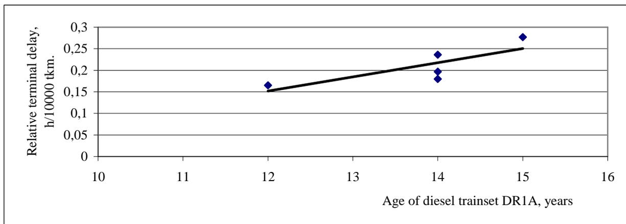
Fig 6. The relationship between relative delay time and age of diesel trainsets
